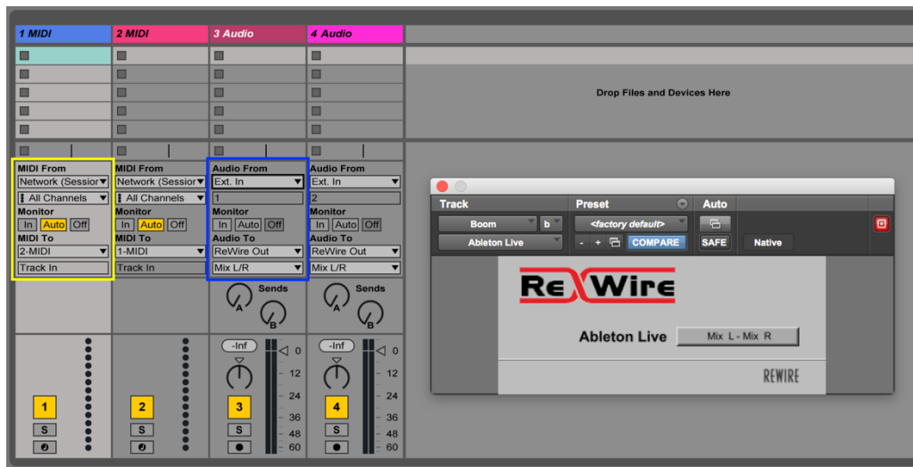
Figure 1.11: Live as ReWire “slave” to Avid’s Pro Tools . The yellow box shows Live receiving MIDI from Pro Tools . The blue box shows Live receiving audio from Pro Tools .
