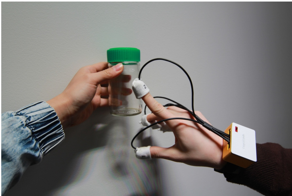
Figure 3.4: “FingerSynth” (2014), created by Gershon Dublon, creates sounds based on the density of objects it touches. [Source: Gershon Dublon and Joseph Paradiso, “FingerSynth: Wearable Transducers for Exploring the Environment with Sound,” Proceedings of the International Conference on New Interfaces for Musical Expression , Goldsmiths, University of London, UK (2014)]
