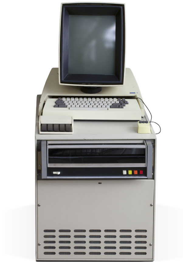
Figure 4.2: Xerox Alto I CPU with monitor, mouse, keyboard and 5-key chording keyset (1973) (Source: Computer History Museum, n.d., accessed April 30, 2016, http://www.computerhistory.org/revolution/input-output/14/347 ).
