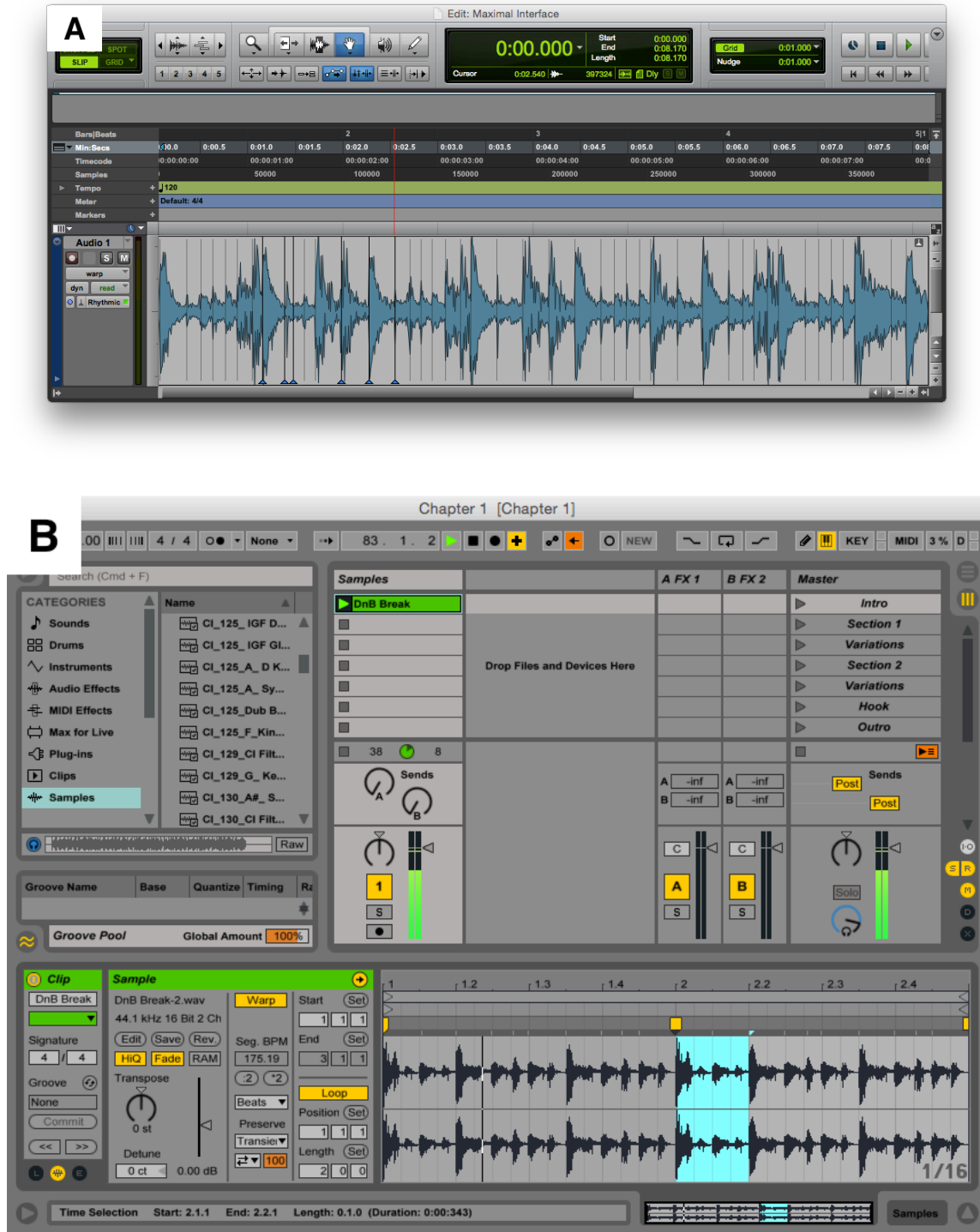
Figure 1.12: “Feature creep” across DAWs. (A) Temporally stretching a sampled drum break using the “Elastic Audio” functionality of Pro Tools 11 . (B) Accomplishing the same task using the audio “Warp” functionality of Live 9 .
