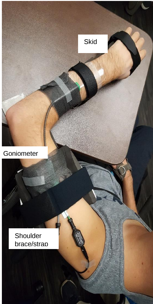
Figure 6.1: Setup of elbow control experiments. (A) Patient resting arm on table, ready for elbow angle to be measured. (B) Electronics setup, patient will follow the angle as viewed in the monitor.
