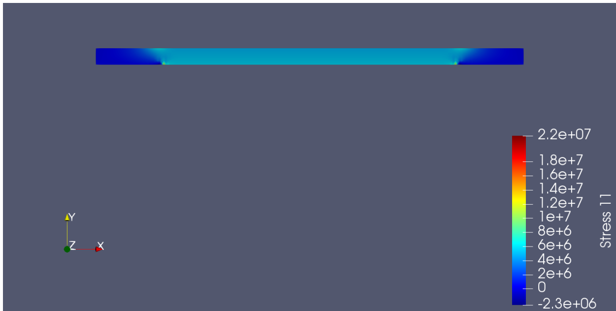
Figure B.4. X-direction stress in the test film at mid-span (linear elastic simulation) at an opening strain of approximately 1.42 mstrain; cross-sectional view. Stress in Pascals.
