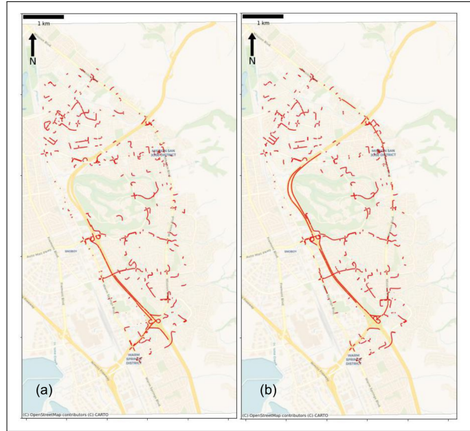
Figure 4.7: Comparison of the spatial distribution of congestion in the Fremont network at 5:30 p.m. showing the congested links (coded red) on the network with \rho = 0.9 . (a): when 40% of the drivers follow dynamic en-route assignment with different thresholds \rho ; (b): when 90% of the drivers follow dynamic en-route assignment.
