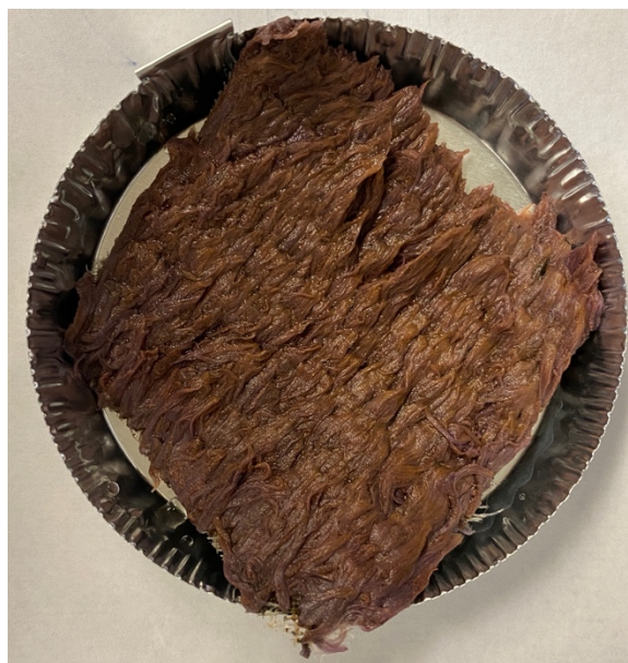
Figure 4 - 2 Cleaned and sonicated cloth tertiary filter
