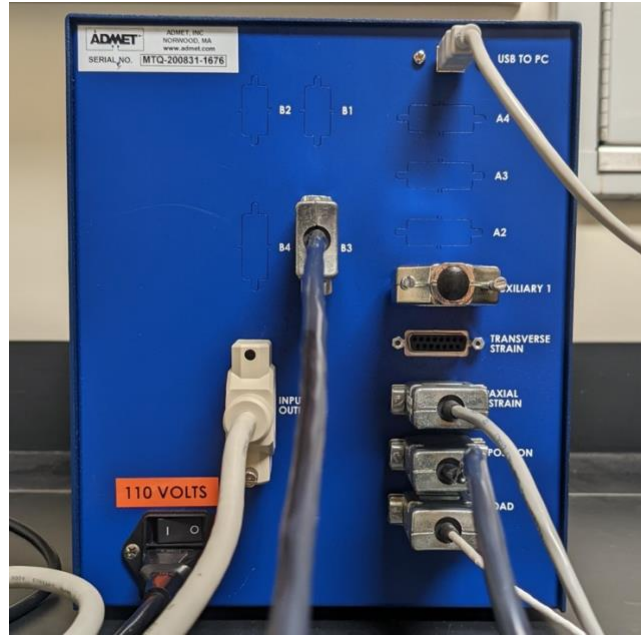
Figure A.5: Back-view of the MTESTQuattro controller box with all the electrical connections attached.
