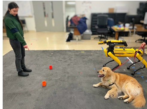
Figure 1: Our system enables a robot to locate objects using information from a person's unscripted gestures. We compare our robot's performance to that of the domestic dog.
