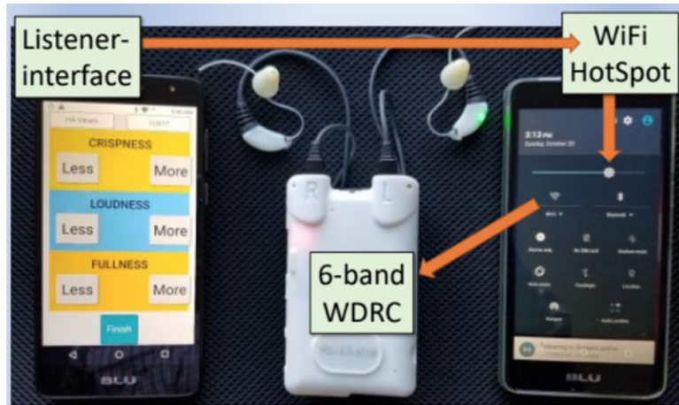
Figure 8: Apparatus used for the SFP study. The arrows represent the information flow from the listener interface, via WiFi, to the Portable OSP to tune the WRDC.
