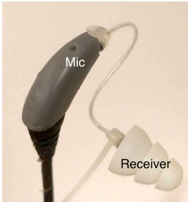
Figure 5: The BTE-RIC hearing aid developed for both the lab-based system and the portable system.
