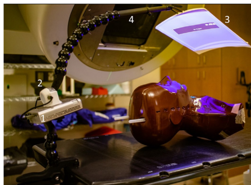
Figure 1 AVATAR system, shown with (1) pico projector, (2) speaker, (3) curved radiolucent screen, and (4) telescopic mount.
