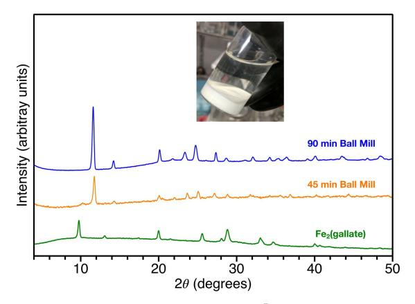
**Figure 4.8:** Powder X-ray diffraction of phase impure  $Fe^{II}(H_2gallate) \cdot 2H_2O$  obtained via 45 minutes of ball milling (orange, middle), possible impurity  $Fe^{II}_2(gallate)$  (green, bottom), and phase pure  $Fe^{II}(H_2gallate) \cdot 2H_2O$  obtained via 90 minutes of ball milling (blue, top) with picture of white 90 min product (inset).
