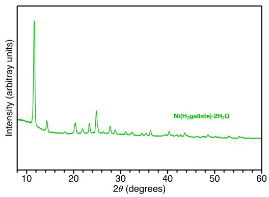
**Figure 4.9:** Powder X-ray diffraction pattern of Ni(H<sub>2</sub>gallate)·2H<sub>2</sub>O obtained via ball milling.
