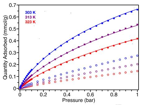
**Figure 3.29:** Comparison of gas adsorption isotherms for  $C_2H_6$  in Fe<sup>II/III</sup>(H<sub>x</sub>gallate) (solid squares) and Fe<sup>II</sup>(H<sub>2</sub>gallate) (empty circles) measured at 303 K (blue, top), 313 K (purple, middle), and 323 K (red, bottom), with multi-site Langmuir-Freundlich fits for Fe<sup>II/III</sup>(H<sub>x</sub>gallate) (solid lines).
