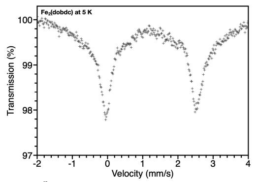
**Figure 2.S14:** <sup>57</sup>Fe Mössbauer spectrum for Fe<sub>2</sub>(dobdc), collected at 5 K. The data (+) could not be fitted to Lorentzian doublets due to superparamagnetic broadening.
