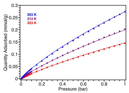
**Figure 3.19:**  $Fe^{II}(H_2gallate) C_2H_6$  gas adsorption isotherms (triangles) measured at 303 K (blue, top), 313 K (purple, middle), and 323 K (red, bottom), with dual-site Langmuir-Freundlich fits (solid lines).
