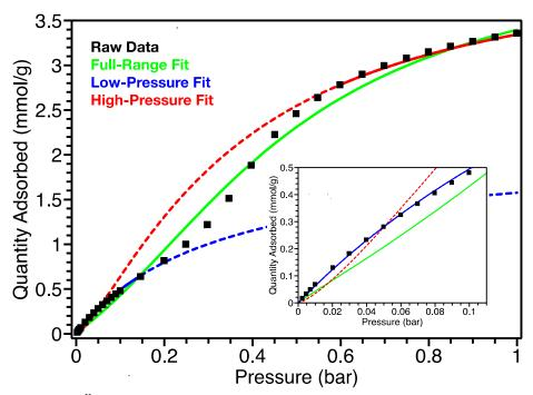
**Figure 3.21:**  $Fe^{II}(H_2gallate) C_2H_4$  gas adsorption isotherm measured at 313 K (black squares), dual-site Langmuir-Freundlich fits for the full pressure range (green solid line), high-pressure range (red solid line), and low-pressure range (blue solid line), with projections in dashed lines and low pressure inset.
