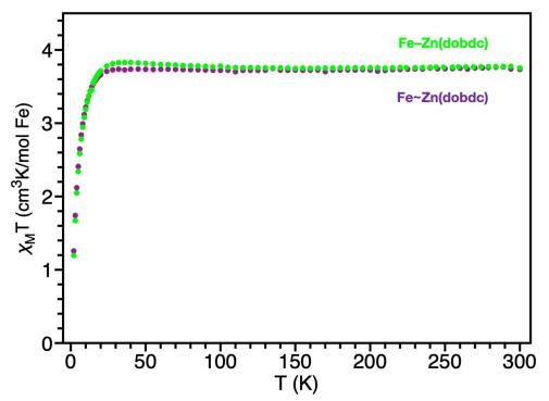
Figure 2.7: Variable-temperature magnetic susceptibility normalized per Fe for Fe-Zn(dobdc) and Fe-Zn(dobdc) collected at 1 kOe
