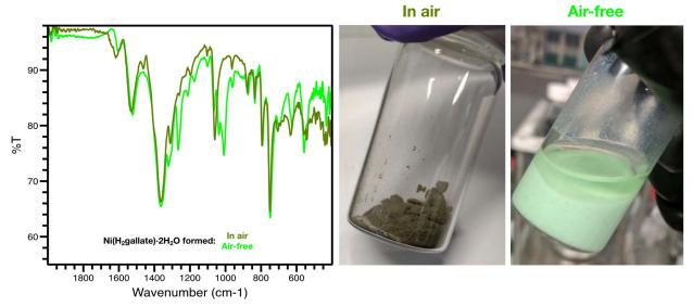
**Figure 4.10:** ATIR spectra (left) for Ni(H<sub>2</sub>gallate)·2H<sub>2</sub>O synthesized via ball milling in air (dark green) and air-free (light green), with pictures of in air synthesized (middle) and air-free synthesized (right).
