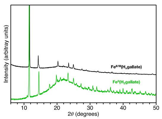
**Figure 3.25:** X-ray powder diffraction pattern of sealed capillaries of activated  $Fe^{II}(H_2gallate)$  (green, bottom) and activated  $Fe^{II/III}(H_xgallate)$  (black, top). There is no observable decrease in symmetry in  $Fe^{II/III}(H_xgallate)$ .
