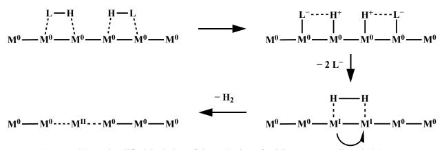
Scheme 4.2: A simplified depiction of the reduction of acidic protons on ligands (L) on a metal surface (M) leading to the formation of  $H_2$  gas. As the metal surface continues to oxide, divalent or higher oxidation state ions dissociate.
