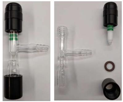
Figure A.1: A  $\frac{1}{2}$ " Breen adapter (left), and the adapter disassembled into its four components (right).
