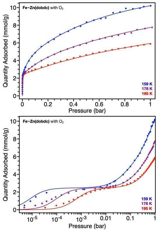
**Figure 2.S4:** Isothermal gas sorption measurement of **Fe~Zn(dobdc)** with O<sub>2</sub> at 159, 178, and 195 K, fitted with a three-site Langmuir-Freundlich equation, parameters found in Table 2.S1, plotted linearly (top) and logarithmically (bottom).
