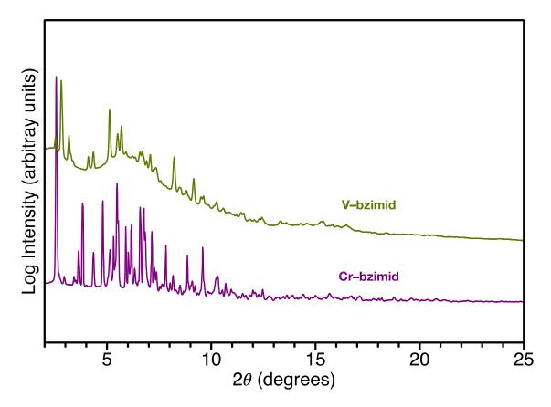
**Figure 4.4:** Powder X-ray diffraction pattern of highly crystalline but phase impure coordination polymers Cr–bzimid (purple, bottom) and V–bzimid (green, top) collected with 0.4972 Å X-rays.
