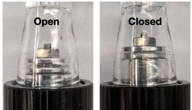
**Figure A.3:** Magnified image of a Breen adapter with a Micromeritics *Transeal* in the open position (left) and the closed position (right).
