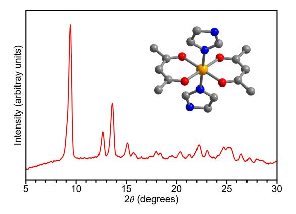
**Figure 4.3:** Powder X-ray diffraction pattern for  $Fe^{II}(acac)_2(Himid)_2$  obtained solvothermally from  $Fe^{III}(acac)_3$  with imidazole in DMF, and structural model of the molecular complex (inset).
