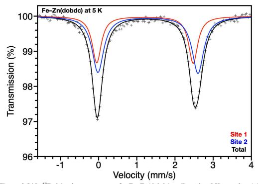
**Figure 2.S10:** <sup>57</sup>Fe Mössbauer spectrum for Fe–Zn(dobdc), collected at 5 K, raw data (+), Site 1 (red), Site 2 (blue), and total fit (black). Parameters for Site 1 and Site 2 found in **Table 2.S4**.
