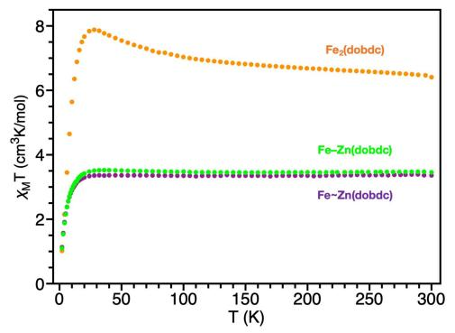
Figure 2.S16: Variable-temperature magnetic susceptibility for  $Fe_2(dobdc)$  collected at 10 kOe and for Fe-Zn(dobdc) and Fe-Zn(dobdc) collected at 1 kOe
