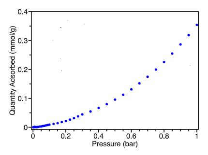
**Figure 3.30:** Gas adsorption isotherms for  $Fe^{II}(H_2gallate)$  in the presence of  $C_2H_6$  at 195 K (blue circles) exhibiting mesoporous condensation.
