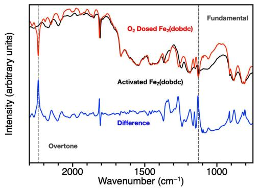
**Figure 2.S8:** DRIFTS measurements of  $Fe_2(dobdc)$  with activated bare framework in black,  $O_2$  dosed in red and the difference spectrum in blue. The fundamental vibrational stretch for superoxide is obscured by framework vibrations but the overtone stretch at 2239 cm<sup>-1</sup> is clearly visible.
