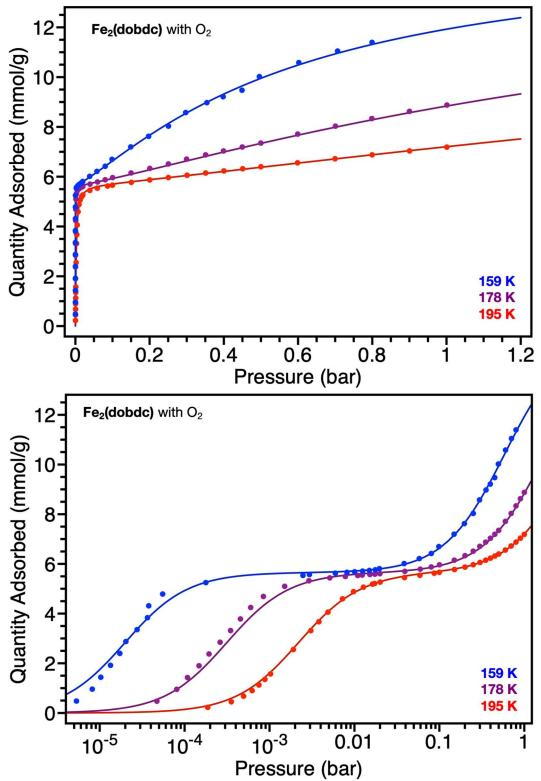
**Figure 2.S6:** Isothermal gas sorption measurement of  $Fe_2(dobdc)$  with O<sub>2</sub> at 159, 178, and 195 K, fitted with a two-site Langmuir-Freundlich equation, parameters found in Table 2.S1, plotted linearly (top) and logarithmically (bottom).
