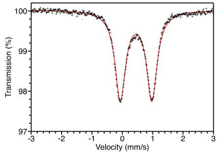
**Figure 3.4:** <sup>57</sup>Fe Mössbauer spectrum for Fe<sup>III</sup>(Hgallate) collected at 290 K (black crosses), consistent with a single high spin Fe<sup>III</sup> site (red line).
