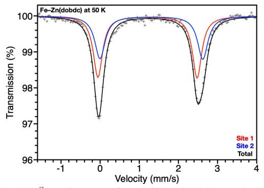
**Figure 2.S9:** <sup>57</sup>Fe Mössbauer spectrum for Fe–Zn(dobdc), collected at 50 K, raw data (+), Site 1 (red), Site 2 (blue), and total fit (black). Parameters for Site 1 and Site 2 found in **Table 2.S4**.
