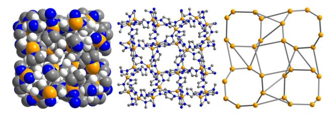
**Figure 4.7:** The highly complex unit cell of the assumed structure of Fe(imid)<sub>2</sub>. A space filling representation (left) shows the visual porosity for a ball and stick model with hydrogens omitted (middle) is nonexistent. A wireframe structure of only metal centers connected to adjacent metal centers (right) reveals the interesting topology of octagonal pores, which are filled by bridging imidazolates.
