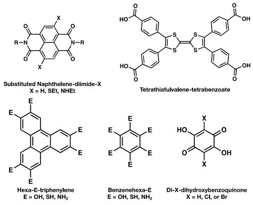
**Figure 1.3:** Example chemical structures of redox-active ligands that have been incorporated into metal–organic frameworks.
