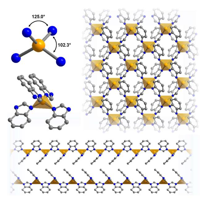
**Figure 4.2:** Single-crystal structure of  $Fe(bzimid)_2$  with hydrogen atoms omitted for clarity. Distorted tetrahedral iron site (top left), coplanar benzimidazolate ligand pairs around an iron center (middle left), view of a single two-dimensional sheet from the *c* axis (top right) and view of herringbone-like stacking of two  $Fe(bzimid)_2$  sheets (bottom).
