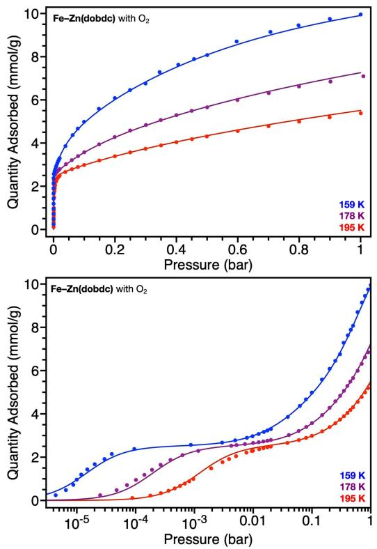
**Figure 2.S2**: Isothermal gas sorption measurement of **Fe–Zn(dobdc)** with O<sub>2</sub> at 159, 178, and 195 K, fitted with a three-site Langmuir-Freundlich equation, parameters found in Table 2.S1, plotted linearly (top) and logarithmically (bottom).
