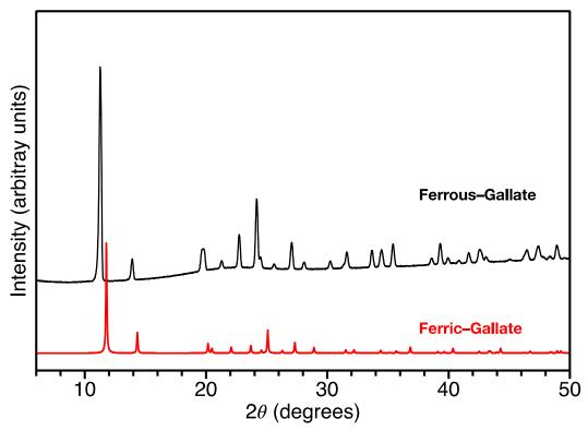
**Figure 3.5:** X-ray powder diffraction pattern of off-white powder presumed to be  $Fe^{II}(H_2gallate)\cdot xH_2O$  (black) matching predicted powder pattern for  $Fe^{III}(Hgallate)\cdot 2H_2O$  (red).
