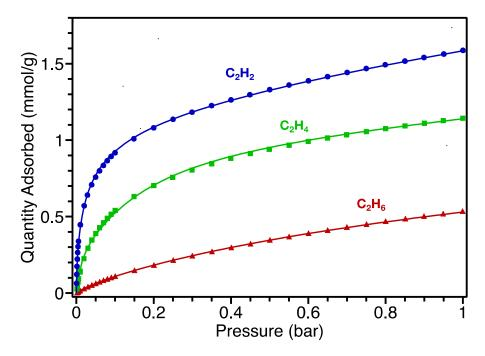
**Figure 3.27:** Example gas adsorption isotherms for  $C_2H_2$  (blue circles),  $C_2H_4$  (green squares), and  $C_2H_6$  (red triangles) in Fe<sup>II/III</sup>(H<sub>x</sub>gallate) at 313 K, fit to multi-site Langmuir-Freundlich isotherms (solid lines).
