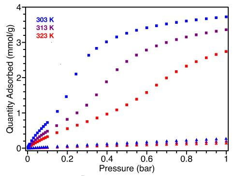
**Figure 3.23:** Comparison of  $\text{Fe}^{II}(\text{H}_2\text{gallate})$  gas adsorption isotherms for  $C_2\text{H}_4$  (squares) and  $C_2\text{H}_6$  (triangles) measured at 303 K (blue, top), 313 K (purple, middle), and 323 K (red, bottom).
