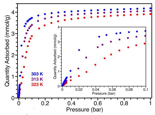
**Figure 3.22:**  $Fe^{II}(H_2gallate) C_2H_2$  gas adsorption isotherms (circles) measured at 303 K (blue, top), 313 K (purple, middle), and 323 K (red, bottom), with low pressure inset.
