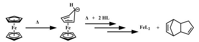
**Scheme 4.1:** The cyclopentadienyl (Cp) ligands in ferrocene can rearomatize when heated to sufficiently high temperature (~150 °C) exposing a highly basic carbanion. This basic species then deprotonates a ligand (L) leading to dissociation of HCp, which readily dimerizes (H<sub>2</sub>Cp<sub>2</sub>). This process is repeated with the other Cp ligand as Fe<sup>2+</sup> ions are eventually incorporated into a coordination solid with L.
