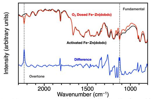
**Figure 2.S7:** DRIFTS measurements of Fe~Zn(dobdc) with activated bare framework in black,  $O_2$  dosed in red and the difference spectrum in blue. The fundamental vibrational stretch for superoxide is obscured by framework vibrations but the overtone stretch at 2233 cm<sup>-1</sup> is clearly visible.
