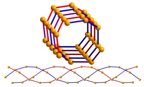
**Figure 4.S1:** Wire-frame representation of an octagonal filled pore in  $Fe(imid)_2$  which has a triple helix structure, with a view down the *c* axis (top) and perpendicular to the *c* axis (bottom). All atoms except Fe are removed and only adjacent metal centers are attached for clarity.
