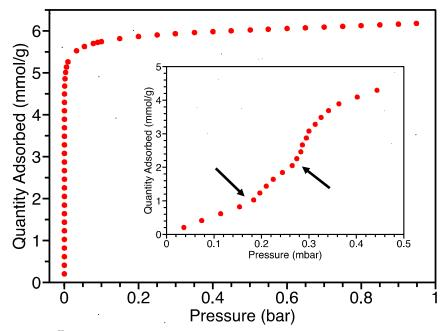
**Figure 3.17:** Fe<sup>II</sup>(H<sub>2</sub>gallate) CO<sub>2</sub> gas adsorption isotherm measured at 195 K with low pressure inset and indicated inflection points consistent with phase changes.
