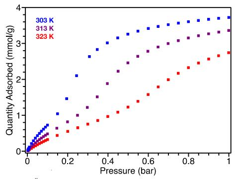
**Figure 3.20:**  $Fe^{II}(H_2gallate) C_2H_4$  gas adsorption isotherms (squares) measured at 303 K (blue, top), 313 K (purple, middle), and 323 K (red, bottom).
