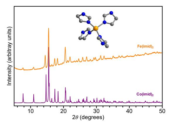
**Figure 4.6:** Comparison of experimentally measured  $Fe(imid)_2$  powder X-ray diffraction pattern (orange, top) with a pattern predicted for  $Co(imid)_2$  (purple, bottom) from a reported single crystal structure,<sup>65</sup> with a representative tetrahedral metal site from the predicted structure of  $Fe(imid)_2$  (inset).
