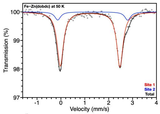
**Figure 2.S11:** <sup>57</sup>Fe Mössbauer spectrum for Fe~Zn(dobdc), collected at 50 K, raw data (+), Site 1 (red), Site 2 (blue), and total fit (black). Parameters for Site 1 and Site 2 found in **Table 2.S4**.
