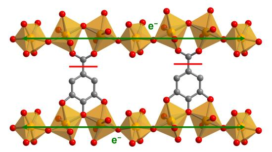
**Figure 3.14:** Crystal structure view of two adjacent vertex sharing iron chains in irongallate. Electronic conductivity is proposed to occur only along these parallel chains (green arrows). Multi-dimensional conductivity is prohibited by the lack of electronic communication between the carboxylate and phenyl ring of the ligand, indicated by red lines.
