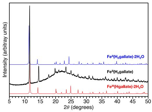
**Figure 3.15:** X-ray powder diffraction pattern of a sealed capillary of activated  $Fe^{II}(H_2gallate)$  (black), compared to predicted patterns for  $Fe^{II}(H_2gallate) \cdot 2H_2O$  (blue) and  $Fe^{III}(Hgallate) \cdot 2H_2O$  (red). New peaks stemming from the reduction in symmetry are visible at 11° and 18°.
