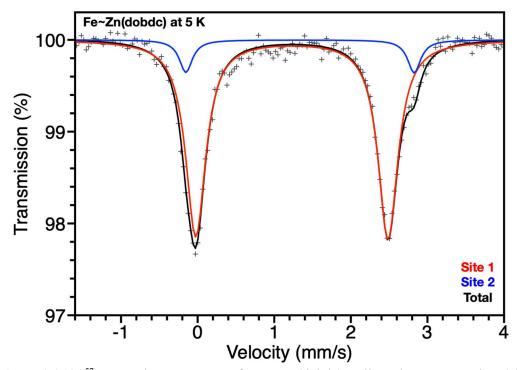
**Figure 2.S12:** <sup>57</sup>Fe Mössbauer spectrum for Fe~Zn(dobdc), collected at 5 K, raw data (+), Site 1 (red), Site 2 (blue), and total fit (black). Parameters for Site 1 and Site 2 found in **Table 2.S4**.
