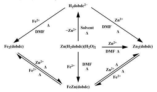
**Scheme 2.1:** There are multiple reactions and equilibria occuring when  $Zn(H_2dobdc)(H_2O)_2$  is heated in DMF in the presence of Fe<sup>2+</sup> cations.
