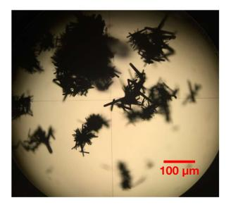
Figure 3.2: Optical microscope image of black needles from iron-gallate screens.
