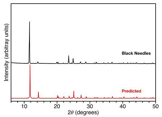
**Figure 3.3:** Powder X-ray diffraction pattern of large black needles from iron–gallate screens (black, top) matching predicted powder pattern for  $Fe^{III}(Hgallate) \cdot 2H_2O$  (red, bottom).
