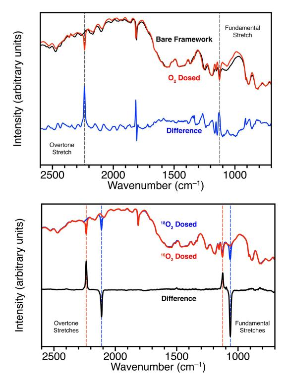
Figure 2.3: (Top) DRIFTS spectra of activated Fe-Zn(dobdc) in black, O<sub>2</sub> dosed Fe-Zn(dobdc) in red, and a difference spectrum in blue. (Bottom) DRIFTS spectra of <sup>16</sup>O<sub>2</sub> dosed Fe-Zn(dobdc) in red, <sup>18</sup>O<sub>2</sub> dosed Fe-Zn(dobdc) in blue, and a difference spectrum in black. Samples were held under 10 mbar O<sub>2</sub> at 195 K.
