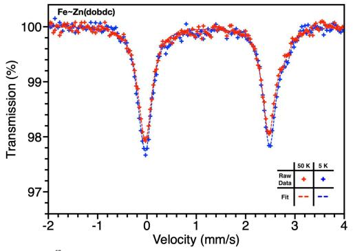
**Figure 2.S15:** <sup>57</sup>Fe Mössbauer spectra for Fe~Zn(dobdc), comparing data from 50 K (red) and 5 K (blue). Similar to Fe–Zn(dobdc), no sign of line broadening is observed.
