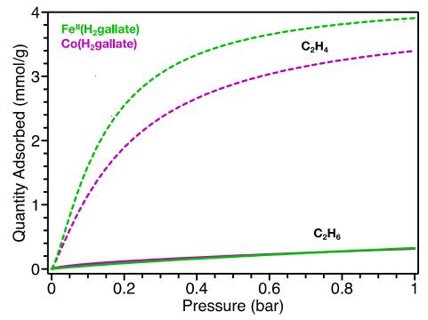
**Figure 3.24:** Modeled dual-site Langmuir-Freundlich isotherms for  $C_2H_4$  (dashed lines) and  $C_2H_6$  (solid lines) in Fe<sup>II</sup>(H<sub>2</sub>gallate) (green) and Co(H<sub>2</sub>gallate) (purple) at 298 K.
