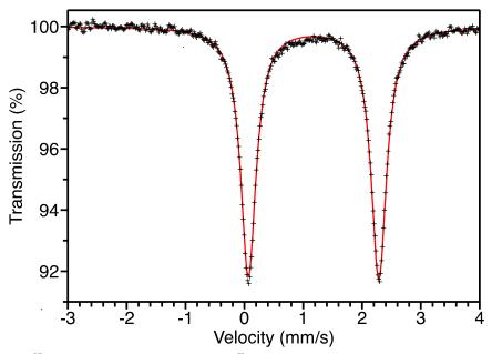
**Figure 3.6:** <sup>57</sup>Fe Mössbauer spectrum for  $Fe^{II}(H_2gallate)$  collected at 295 K (black crosses), consistent with a single high spin  $Fe^{II}$  site (red line).
