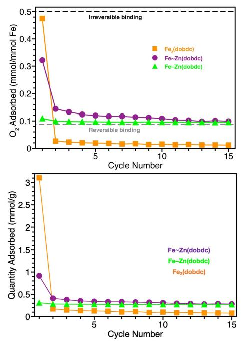
Figure 2.9:  $O_2$  adsorption cycling measurements for  $Fe_2(dobdc)$  (orange squares),  $Fe \sim Zn(dobdc)$  (purple circles, and Fe - Zn(dobdc) (green triangles). Scaled by Fe content (mmol/mmol Fe) (top) with expected one-time irreversible uptake for peroxide formation (black dashed line) and expected fully reversible uptake for superoxide formation (grey dashed line) and plotted in mmol/g (bottom).
