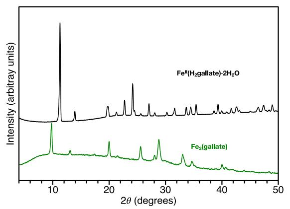
**Figure 3.S1**: Comparison of powder X-ray diffraction patterns of  $Fe_2(gallate)$  (green, bottom), vs  $Fe^{II}(H_2gallate) \cdot 2H_2O$  (black, top).  $Fe_2(gallate)$  was obtained as a green powder from the reaction of stoichiometric equivalents of  $FeCl_2$  and gallic acid in a 3:1 DMF:H<sub>2</sub>O solution in a sealed tube at 120 °C for 1 day.
