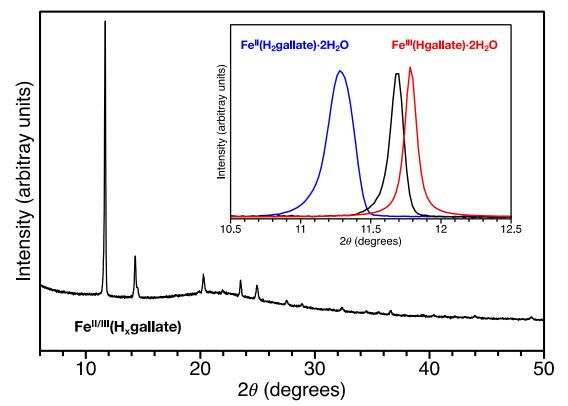
**Figure 3.12:** X-ray powder diffraction pattern of  $Fe^{II/III}(H_xgallate)$  (black), with inset comparing the position of the first diffraction peak to those of  $Fe^{II}(H_2gallate) \cdot 2H_2O$  (blue) and  $Fe^{III}(Hgallate) \cdot 2H_2O$  (red).
