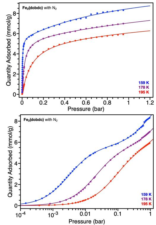
**Figure 2.S5:** Isothermal gas sorption measurement of  $Fe_2(dobdc)$  with N<sub>2</sub> at 159, 178, and 195 K, fitted with a two-site Langmuir-Freundlich equation, parameters found in Table 2.S1, plotted linearly (top) and logarithmically (bottom).
