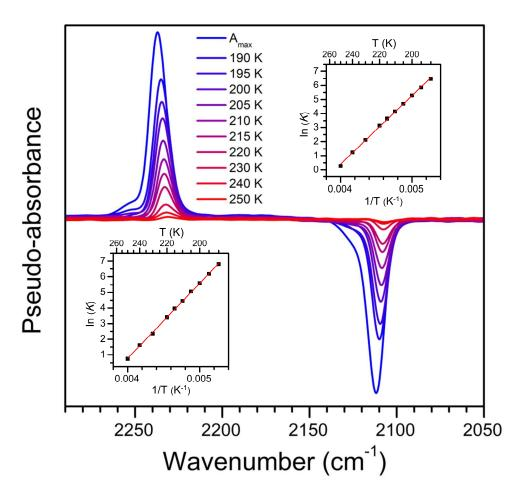
**Figure 2.4:** Variable temperature difference DRIFTS spectra of superoxide overtone stretch for <sup>16</sup>O<sub>2</sub> dosed **Fe–Zn(dobdc)** (top left, positive peaks) and <sup>18</sup>O<sub>2</sub> dosed **Fe–Zn(dobdc)** (bottom right, negative peaks). Van't Hoff plot insets for equilibrium data comparing peak area to maximum measure for <sup>16</sup>O<sub>2</sub> (bottom left inset) and <sup>18</sup>O<sub>2</sub> (top right inset).
