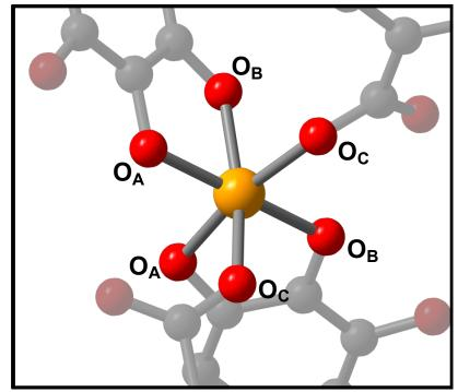
Figure 3.10: Single metal site in iron–gallate with oxygen atoms labeled for reference to Table 3.1: bridging middle phenol ( $O_A$ ), terminal side phenol ( $O_B$ ), carboxylate ( $O_C$ ). Adjacent metal sites omitted for visual clarity.
