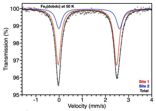
**Figure 2.S13:** <sup>57</sup>Fe Mössbauer spectrum for Fe<sub>2</sub>(dobdc), collected at 50 K, raw data (+), Site 1 (red), Site 2 (blue), and total fit (black). Parameters for Site 1 and Site 2 found in **Table 2.S4**.
