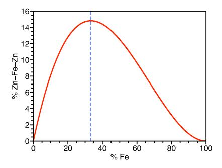
**Figure 2.2:** For a material  $Fe_{2x}Zn_{2(1-x)}(dobdc)$  with completely random distribution, the probability of desired metal distribution Zn–Fe–Zn is calculated as  $(1-x)\times(x)\times(1-x)$ , shown in red. The maximum would occur at 1:2 Fe:Zn (dotted blue line).
