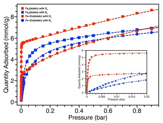
**Figure 2.5:** Gas Sorption isotherms of  $Fe_2(dobdc)$  (squares) and  $Fe_Zn(dobdc)$  (circles) for O<sub>2</sub> (red) and N<sub>2</sub> (blue) at 178 K with low pressure region magnified (inset). Multisite Langmuir-Freundlich fits from simultaneously fitting multiple temperatures are shown as dashed lines.
