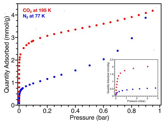
**Figure 3.26:** Gas adsorption isotherms for  $N_2$  at 77 K (blue circles, bottom) and  $CO_2$  (red circles, top) in Fe<sup>II/III</sup>(H<sub>x</sub>gallate) with no discernable low-pressure phase change.
