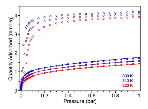
**Figure 3.31:** Comparison of gas adsorption isotherms for  $C_2H_2$  in Fe<sup>II/III</sup>(H<sub>x</sub>gallate) (solid squares) and Fe<sup>II</sup>(H<sub>2</sub>gallate) (empty circles) measured at 303 K (blue), 313 K (purple), and 323 K (red), with multi-site Langmuir-Freundlich fits for Fe<sup>II/III</sup>(H<sub>x</sub>gallate) (solid lines).
