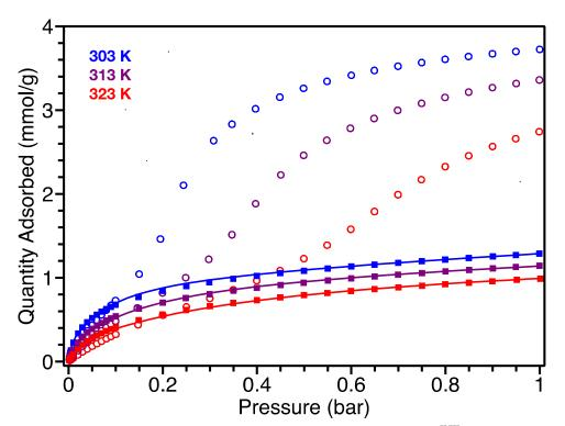
**Figure 3.28:** Comparison of gas adsorption isotherms for  $C_2H_4$  in Fe<sup>II/III</sup>(H<sub>x</sub>gallate) (solid squares) and Fe<sup>II</sup>(H<sub>2</sub>gallate) (empty circles) measured at 303 K (blue), 313 K (purple), and 323 K (red), with multi-site Langmuir-Freundlich fits for Fe<sup>II/III</sup>(H<sub>x</sub>gallate) (solid lines).
