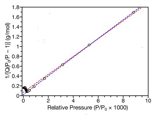
**Figure 3.18:** BET fit of low-pressure region of  $Fe^{II}(H_2gallate)$  195 K CO<sub>2</sub> isotherm (empty black circles), with fit of the entire low-pressure region including phase transitions (red dashed line) and fit excluding the phase transitions (blue dashed line). Q: quantity adsorbed, P: Pressure, P<sub>0</sub>: saturation pressure of CO<sub>2</sub> at 195 K.
