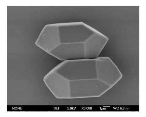
**Figure 3.7:** Scanning electron microscopy image of single crystals of  $Fe^{II}(H_2gallate) \cdot 2H_2O$ , exhibiting clearly defined facets consistent with a pentagonal dodecahedron elongated along a 3-fold axis.
