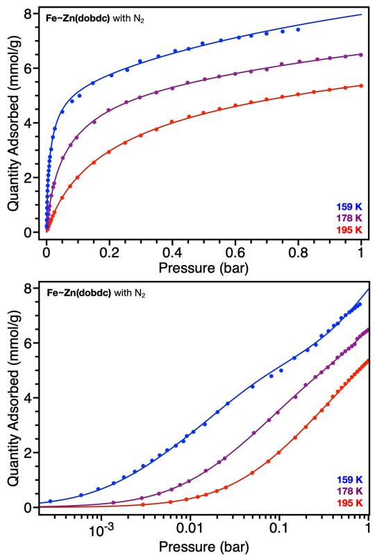
**Figure 2.S3:** Isothermal gas sorption measurement of **Fe~Zn(dobdc)** with N<sub>2</sub> at 159, 178, and 195 K, fitted with a three-site Langmuir-Freundlich equation, parameters found in Table 2.S1, plotted linearly (top) and logarithmically (bottom).
