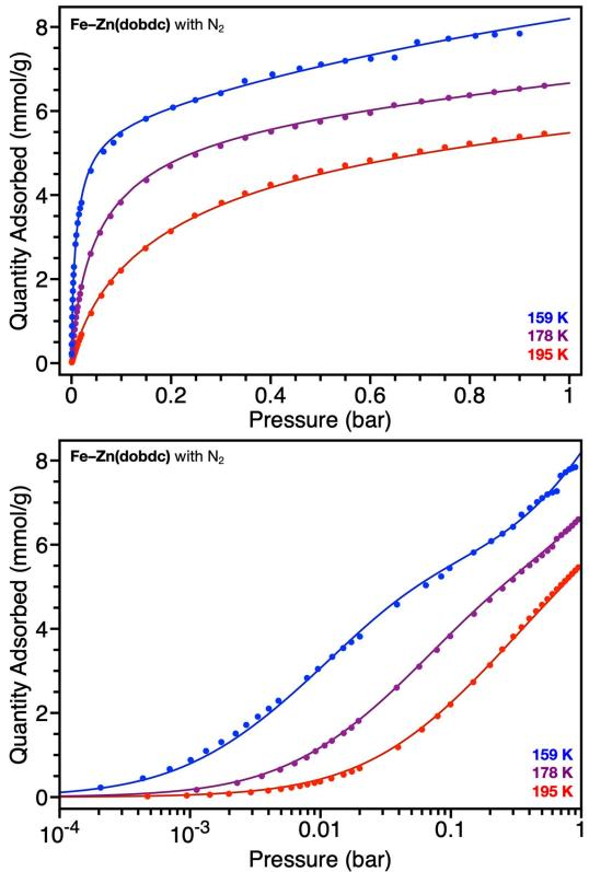
**Figure 2.S1**: Isothermal gas sorption measurement of Fe-Zn(dobdc) with N<sub>2</sub> at 159, 178, and 195 K, fitted with a three-site Langmuir-Freundlich equation, parameters found in Table 2.S1, plotted linearly (top) and logarithmically (bottom).
