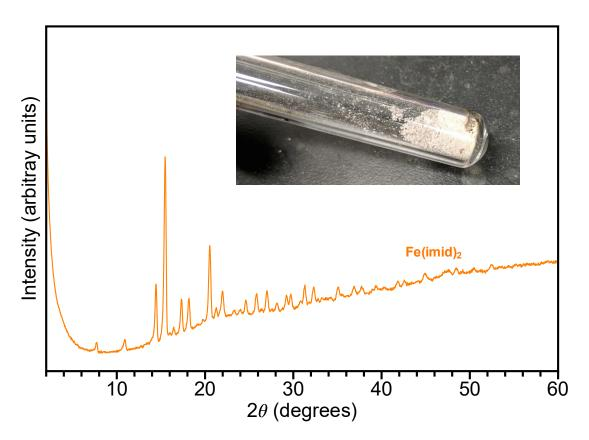
**Figure 4.5:** Powder X-ray diffraction pattern for  $Fe(imid)_2$  obtained as a voluminous white powder (inset) via a minimalist reaction.
