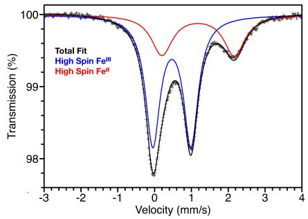
**Figure 3.13:** <sup>57</sup>Fe Mössbauer spectrum for  $Fe^{II/III}(H_xgallate)$  collected at 295 K (grey crosses) fit to two sites: high spin  $Fe^{III}$  (blue line), high spin  $Fe^{II}$  (red line), and total fit (black line).
