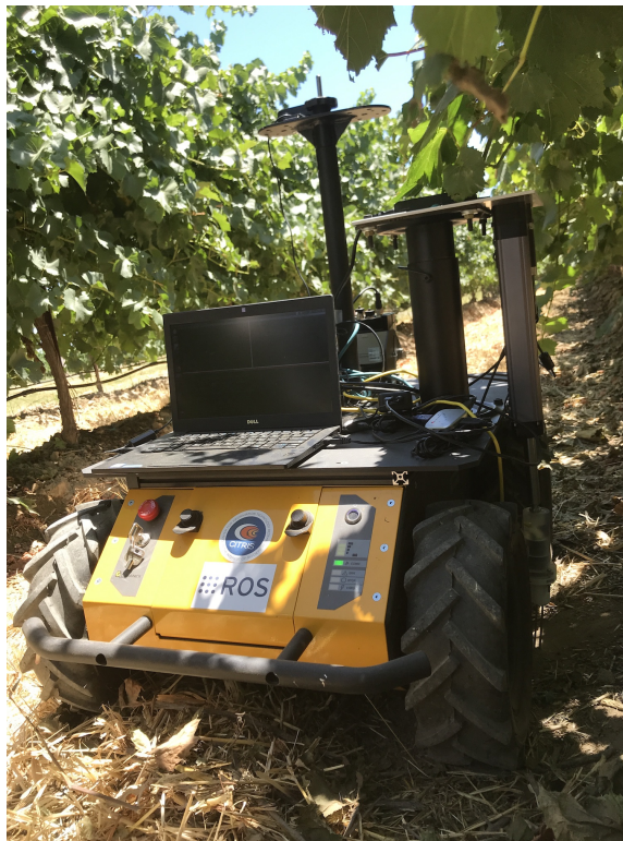
Figure 5.1: A prototype robot built with the Clearpath Husky platform and equipped with a linear actuator mounted soil moisture probe connected to a data logger.
