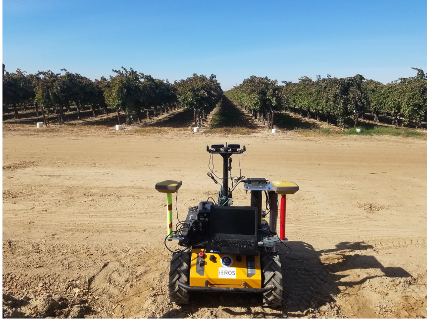
Figure 4.1: A Clearpath Husky robot next to a vineyard located in Central California. The distance between rows is clearly visible and demonstrates how little room there is for maneuverability of multiple robots.
