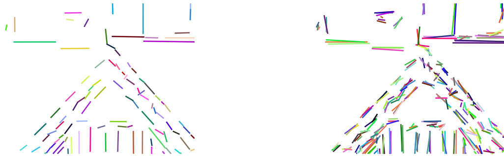
Figure 4.8. Line segment perturbation. In addition to the originally detected line segments, we intentionally duplicate each one d times while randomly perturbing its endpoints within \pm 3 pixels. By doing so, we blur the DUDE descriptors and make them less sensitive to unstable endpoint detection.
