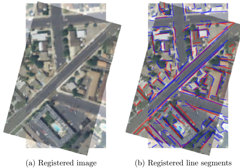
Figure 3.9. (a) shows the registration result using the optimal transformation T^* . (b) visualizes how S and S' are finally matched.
