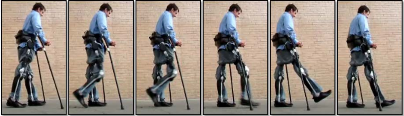
Figure 3-8: Swing Sequence of the Ryan Exoskeleton
