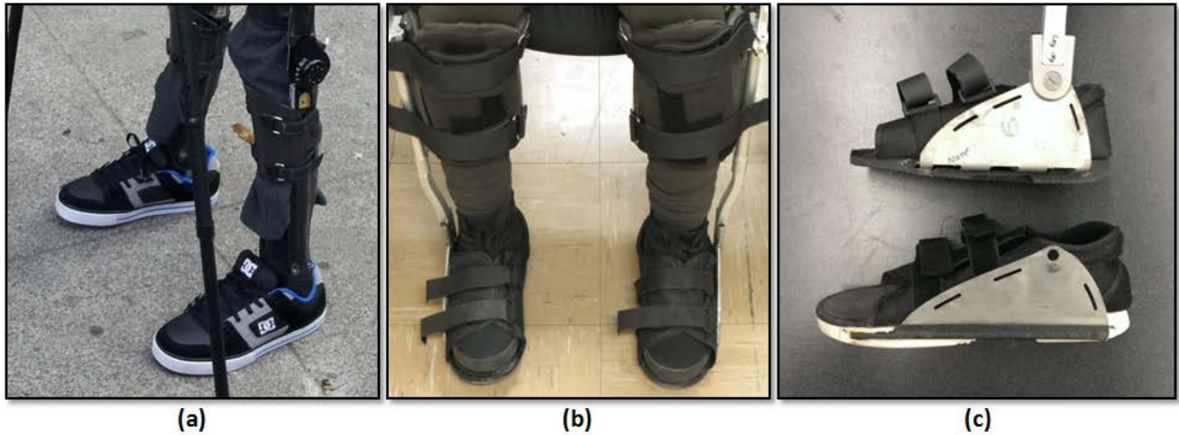
Figure 3-17: (a) Internal Foot Interface (b) External Exoskeleton Shoes (c) Sizes Large and Small
