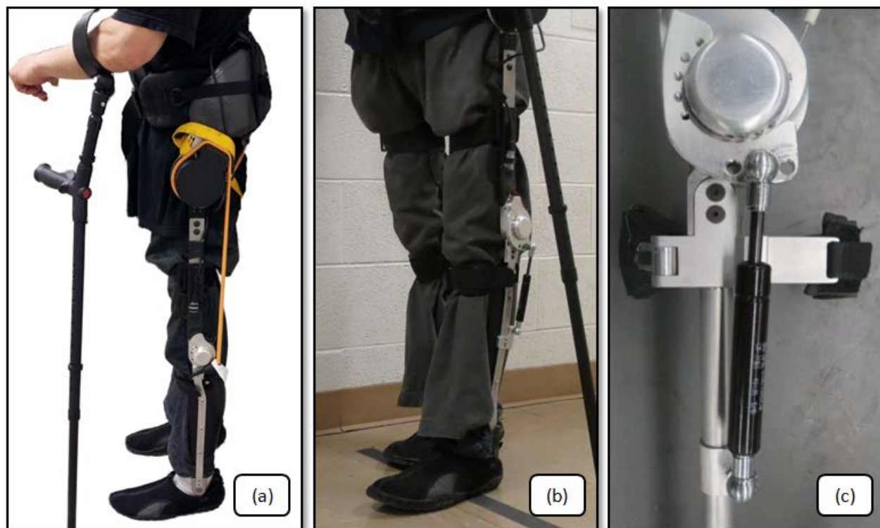
Figure 3-12: (a) Preliminary Swing-Extension Energy Capture Setup (b) Knee Spring Damper Add-on (c) Close-up view
