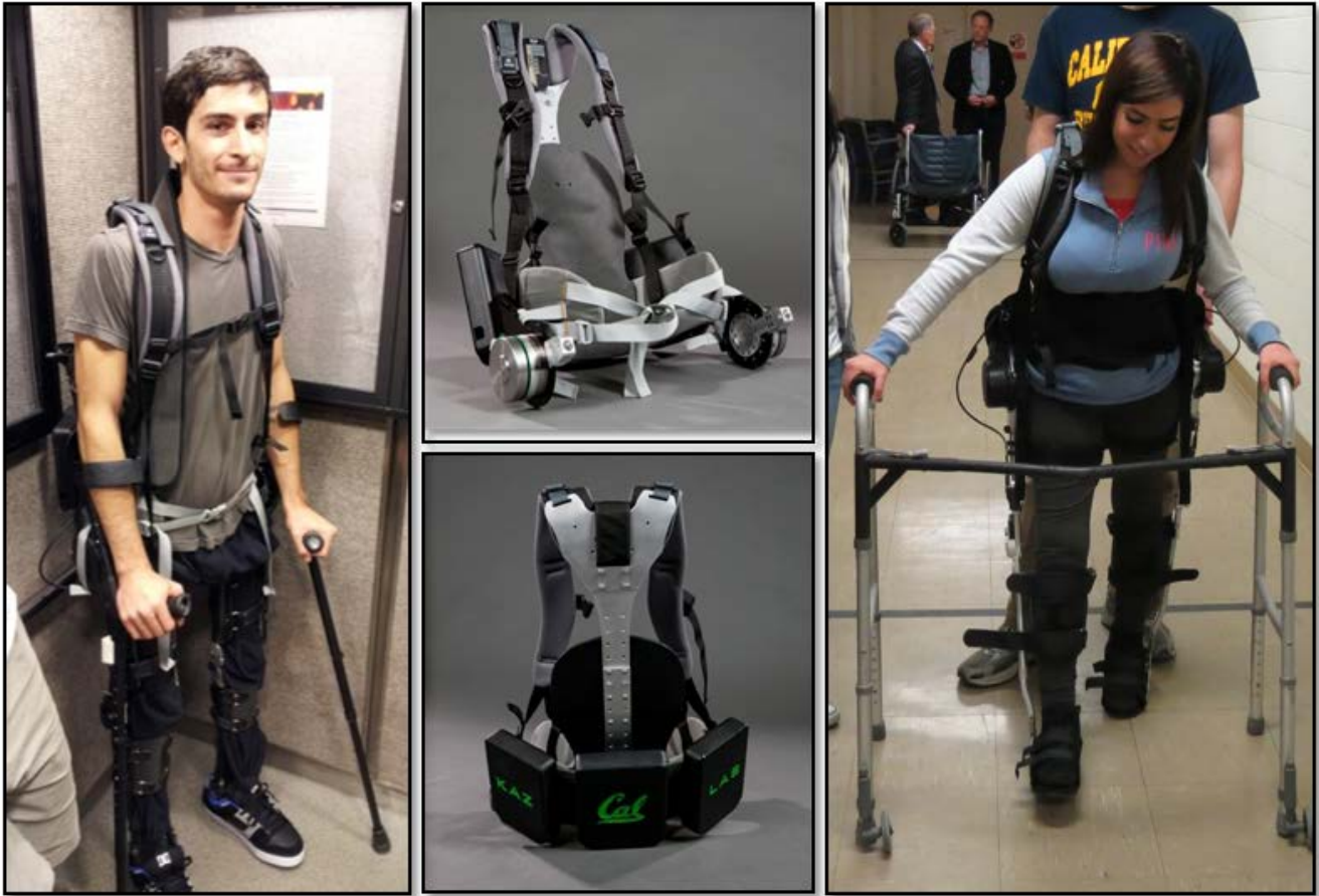
Figure 3-13: Extended Torso Frame for the Ryan Exoskeleton (Left) Demonstration of use of the corset and walker (Right)
