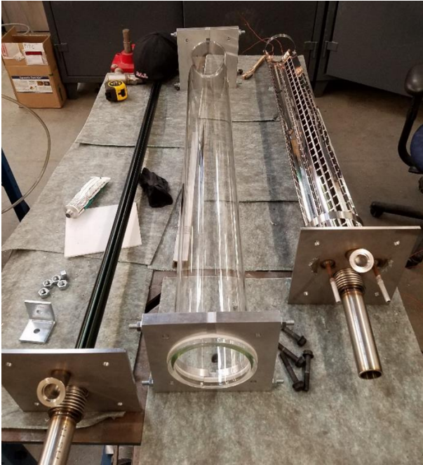
Figure 5.34 – (above) 3-piece assembly for the Hybrid HCE. Step 1-insert secondary reflector/end cap and secure to glass tube. Step 2-insert absorber/end cap from other side and secure to glass tube. Make cell connections and weld absorber. The fully assembled hybrid HCE is pictured on the right.
