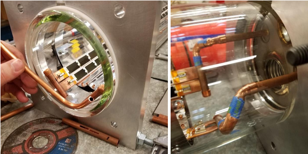
Figure 5.27 – Minichannel connections at U-bend (left) and cap end (right).
