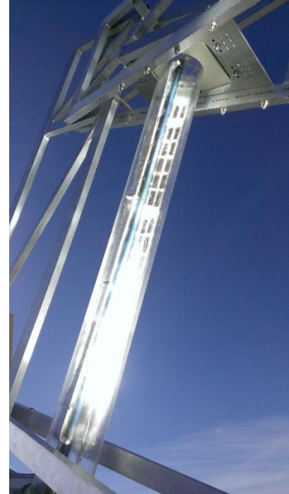
Condensation causes significant reflection / scattering when illuminated
