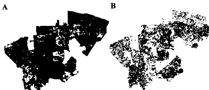
Figure 4.16: The unclassified image of Hod HaSharon is in panel A. The classified image is in panel B. The red pixels represent built land uses, beige represent bare and undeveloped land uses, and the gray represent areas outside of the city borders.
