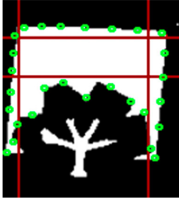
Figure 5.9: Shows edge point traces of outward stencil scan.
