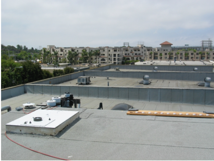
Figure 4.14: Roof platform at Biospherical Instruments, Inc with the top of the SUV-100 spectroradiometer on the left side and the board with all UV sensors on the right side. The collector of the SUV-100 spectroradiometer is the round object protruding the white box, which contains the SUV-100 instrument.
