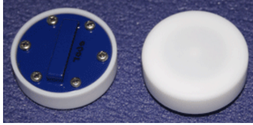
Figure 4.9: Digital UVB dosimeter manufactured by NIWA used for our extended experiments estimating body site UV exposure. One of the sensors used in our experiments.
