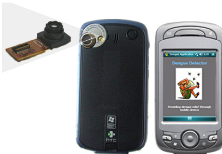
Figure 5.6: HTC Mogul 6800 cellular platform with embedded optical sensor.
