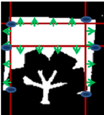
Figure 5.8: Shows gradient points marked from each respective scan and stencil scan to define the edge. The blue circle represents a strong gradient point, G_i(x,y) , that forms a line segment cutting through patch. The green arrow represents the stencil scan direction to the approximate edge of the patch.
