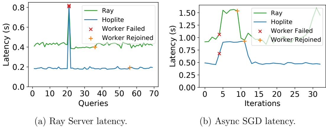
Figure 2.12: Latency when a participating task fails and rejoins on (a) Ray Serve and (b) async SGD.
