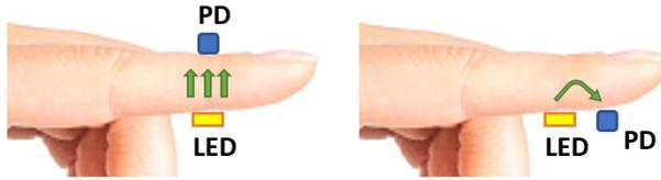
Figure 1.1: Schematics of PPG sensor design
