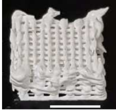
Figure S1.1. Failed woodpile printed at 69 kPa with 410 μm nozzle diameter. Scale bar: 5 mm.
