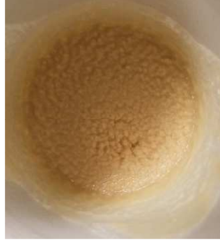
Figure 5.1. Bioink containing 30w/v% AAM inside the cup after mixing for 1min in the planetary mixer. The agglomerates are present at the surface of the ink which are not present in properly mixed ink.
