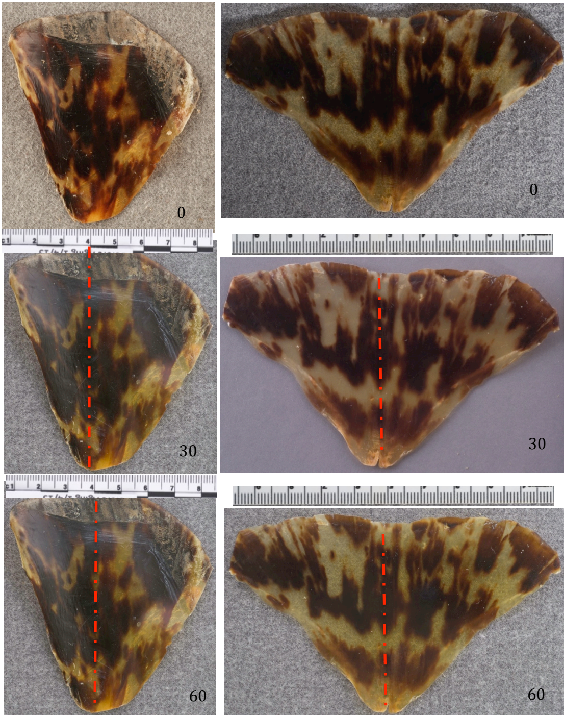
Figure 41. Costal scute 4 dorsal view (left) and Vertebral scute 1 dorsal view (right) at 0, 30, and 60 days of aging in the UVA chamber, photographed in diffuse light (aged sides are to the right of dashed line). Both scutes show a visible shift to yellow in light areas, surface matting, and dulling of the dark melanized regions.
