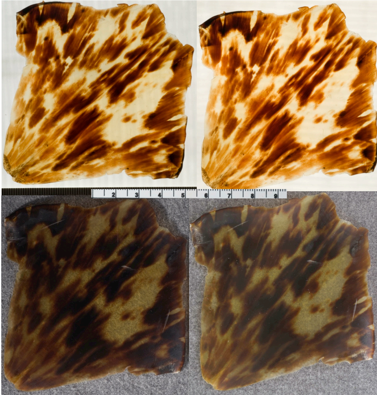
Figure 53. Top: Photographs of dorsal side V3 (aged in museum chamber) in transmitted light, before aging (left) and after 60 days aging (right). Bottom: V3 photographed in diffuse light before aging (left) and after 60 days aging (right), for comparison of the two techniques. Transmitted light photography is useful for documenting the translucency of the tortoiseshell and the density of the melanin, however it does not reveal information about the moiré patterning and it was not helpful for revealing visual changes after aging (the diffuse light images were more revealing of change).
