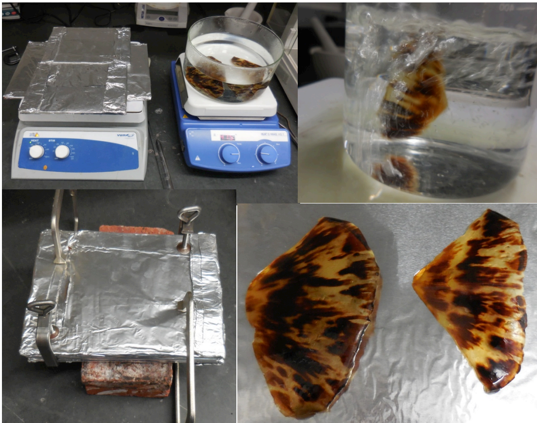
Figure 37. Procedure for flattening the scutes by heating them in boiling water, then applying pressure by placing them between steel plates and clamping them until cool.
