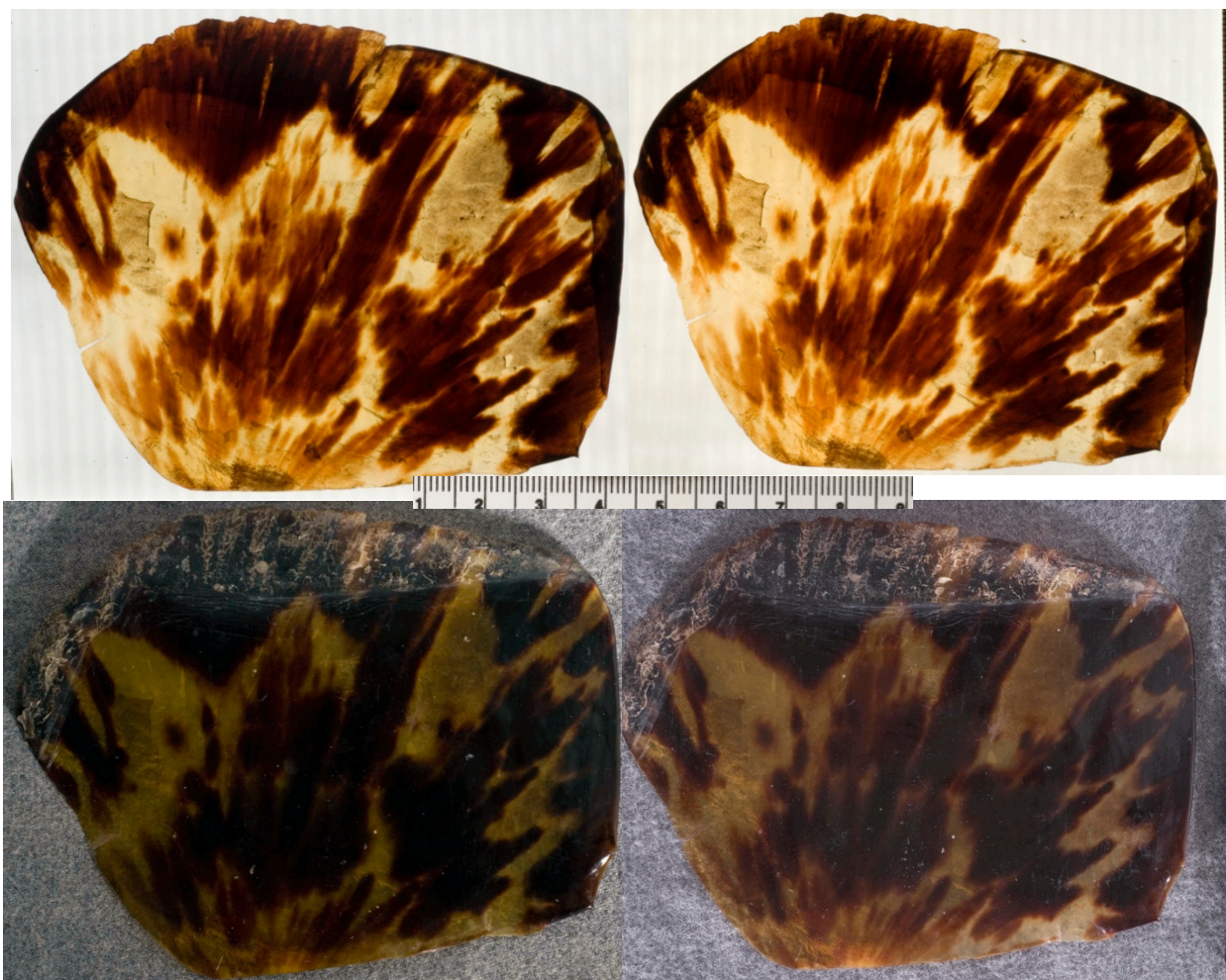
Figure 52. Top: Photographs of C3 (aged in window chamber) in transmitted light, before aging (left) and after 60 days aging (right). Bottom: Dorsal side of C3 photographed in diffuse light before aging (left) and after 60 days aging (right), for comparison of the two techniques. Transmitted light photography is useful for documenting the translucency of the tortoiseshell and the density of the melanin, however it does not reveal information about the moiré patterning and it was not helpful for revealing visual changes after aging.
