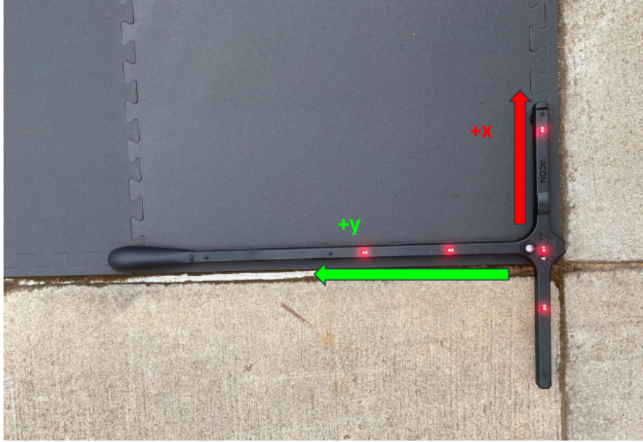
Figure 5.5. Vicon Wand Defining The World Origin. Short end of wand determines the x-axis, long handle points in the positive y-axis direction. Following the right hand rule, positive z is up from the ground, in the direction of the IR sensors.
