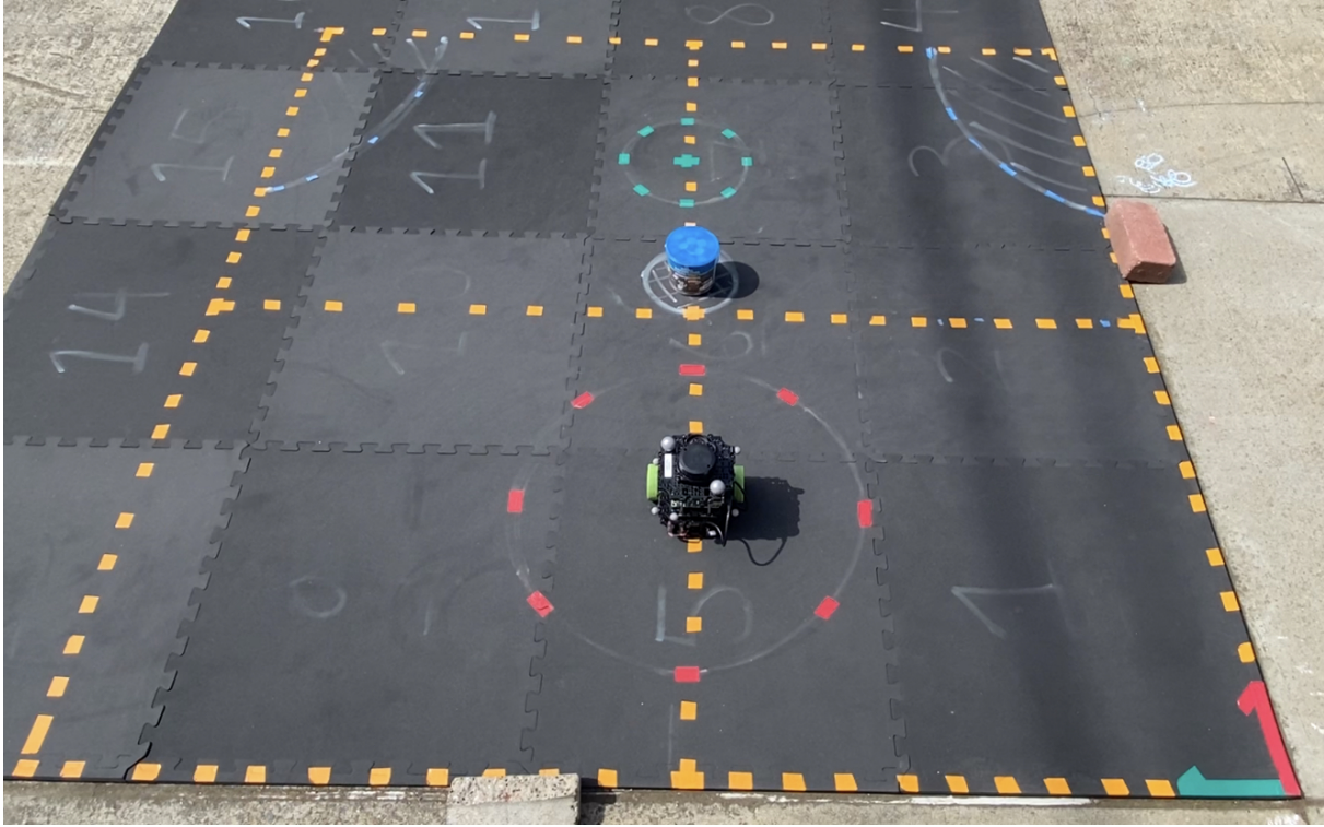
Figure 5.2. Hardware Setup. A black mat was laid out within the UCSD aerodrome which contains 30 IR cameras. The orange dotted lines represent 1 meter by 1 meter squares. The positive y-axis is in the direction of the green arrow at the bottom right and the positive x-axis the red. The Turtlebot3 Burger is the black wheeled robot within the red circle. The red circle represents the 0-levelset of the initial candidate CBF. The final obstacle set is represented by the blue lines and chalk bucket in the center. The green circle represents the goal set \mathcal{G} .
