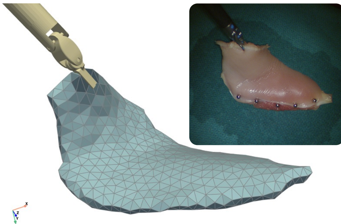
Figure 4.1. The insertion-shaft on surgical robotic tools is an excellent feature for localization. In this work, we present a novel approach for detecting the insertion-shaft and incorporating it into Bayesian filtering to probabilistically localize and track surgical robotic tools. We stress test our method in a challenging deformable tissue dataset where a surgical robotic tool is in the back of the scene with low light and commanded to deform tissue. The tissue is registered to a simulated scene using a separate approach in the camera frame [95] and notice how well aligned the grasp between the localized surgical robotic tool and the tissue is in the 3D rendering.
