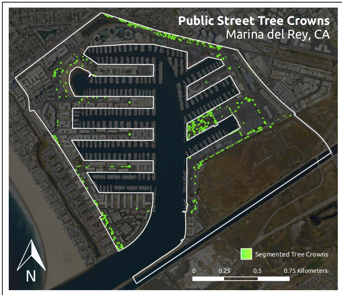
Figure 10. Individual tree crowns for Marina del Rey, CA processed using the raster-based Dalponte2016 tree crown delineation algorithm with CHM inputs derived from LARIAC 4 LiDAR data.
