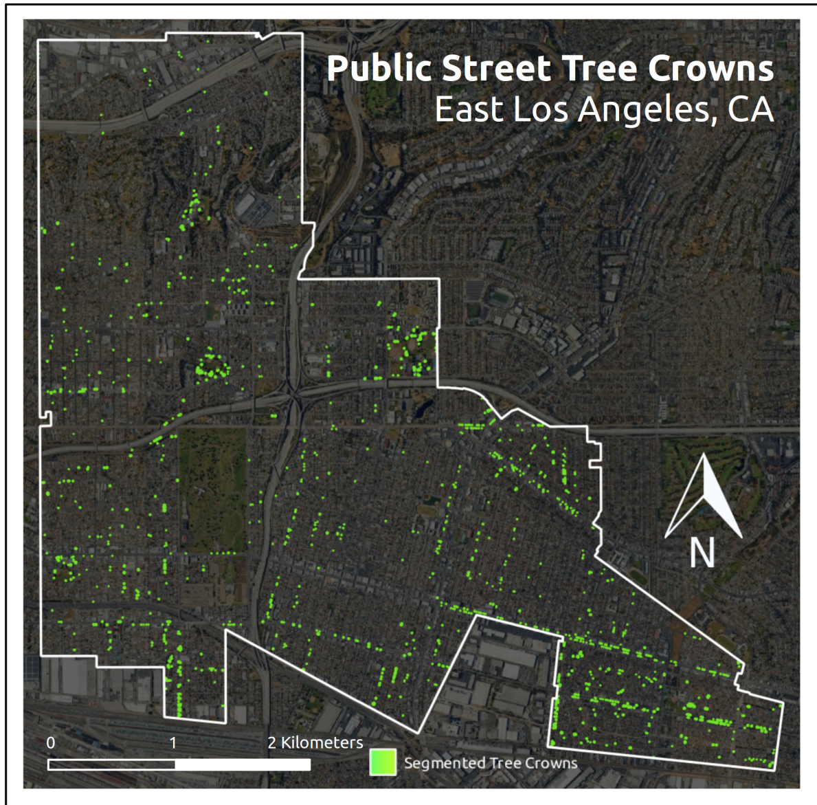
Figure 9. Individual tree crowns for East Los Angeles, CA processed using the raster-based Dalponte2016 tree crown delineation algorithm with CHM inputs derived from LARIAC 4 LiDAR data.
