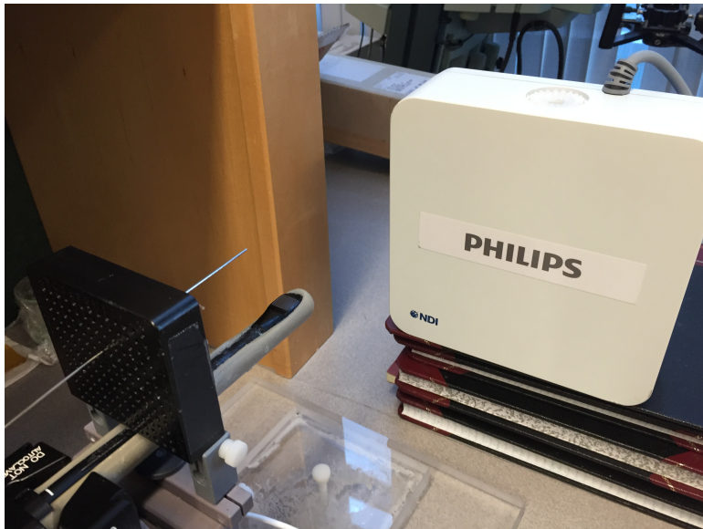
Figure 4: Brachytherapy system, including stylet, ultrasound probe, and field generator in laboratory environment. EM probes are located underneath the transducer head, 5 mm from the distal end of the stylet, and below the template grid.
