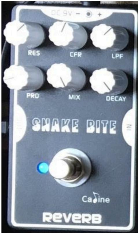
frequency is set by adjusting the middle knob. The rightmost knob is a Low Pass Filter, which alters the timbre of the reverb response.
