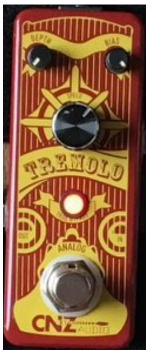
The purpose of this pedal is to add movement to the sound. The main knob in the middle controls the speed of the tremolo. As the knob moves counter-clockwise, the speed gets slower. The speed gets faster as the knob turns in a clockwise direction.
