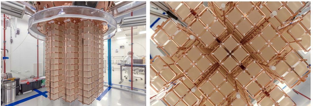
Figure 4. Two pictures of the CUORE detector after its installation in August 2016. Left: a picture of the detector attached to the MSP inside the CUORE cryostat cleanroom. Right: a bottom view of the 19 CUORE towers.
