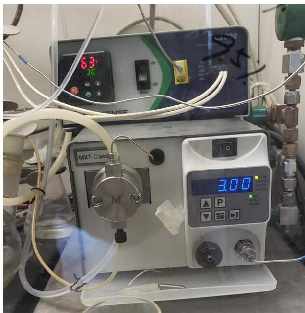
Figure A1.4 Pump and temperature controller
