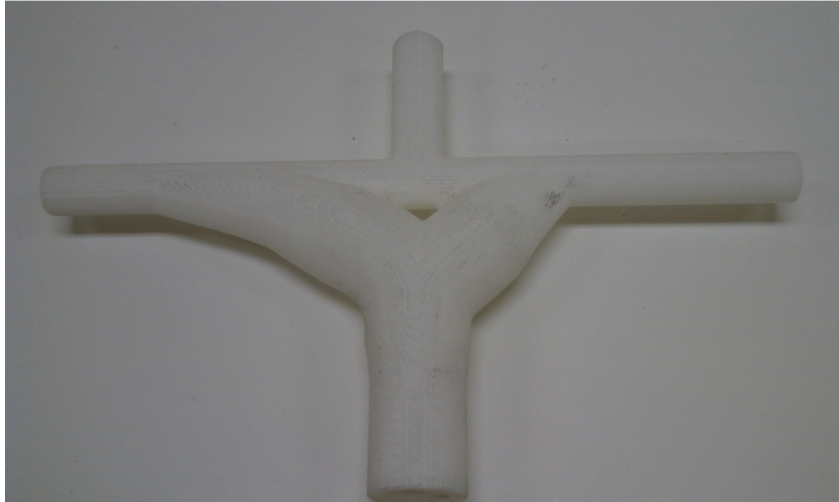
Figure 5. ABS plastic model printed using 3D printer.
