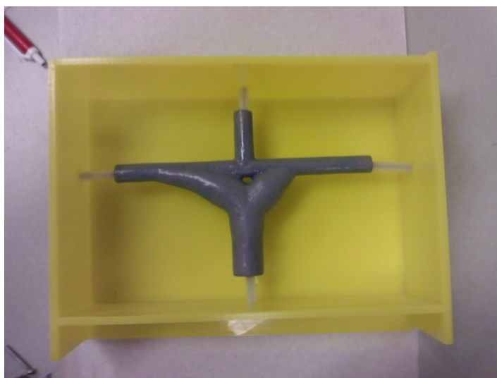
Figure 9. Model coated in primer and glue and suspended in acrylic box.
