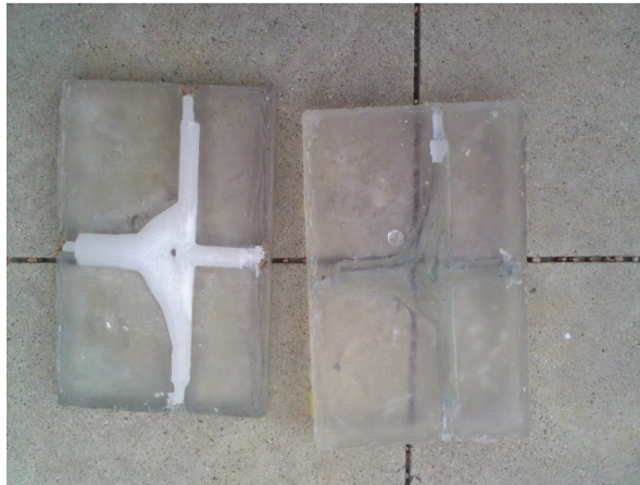
Figure 6. Resin model with wax model inside.
