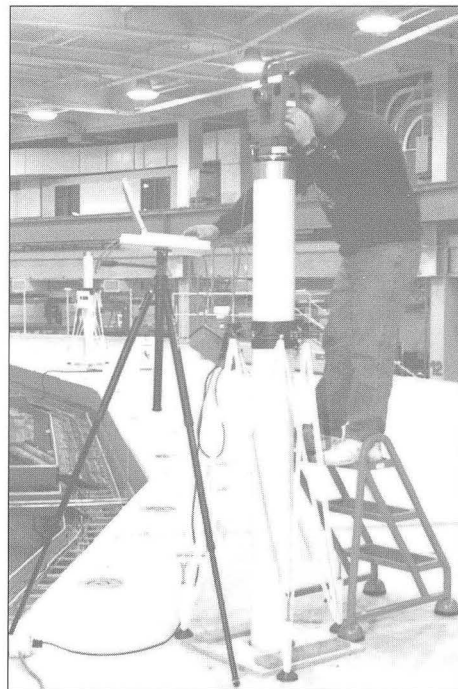
Alex Gavidia sights from one monopod to another atop the storage-ring shielding. The monopod extends through the shielding to a monument set in the floor under the storage ring; shorter ones are used for measurements made from the experiment floor.
