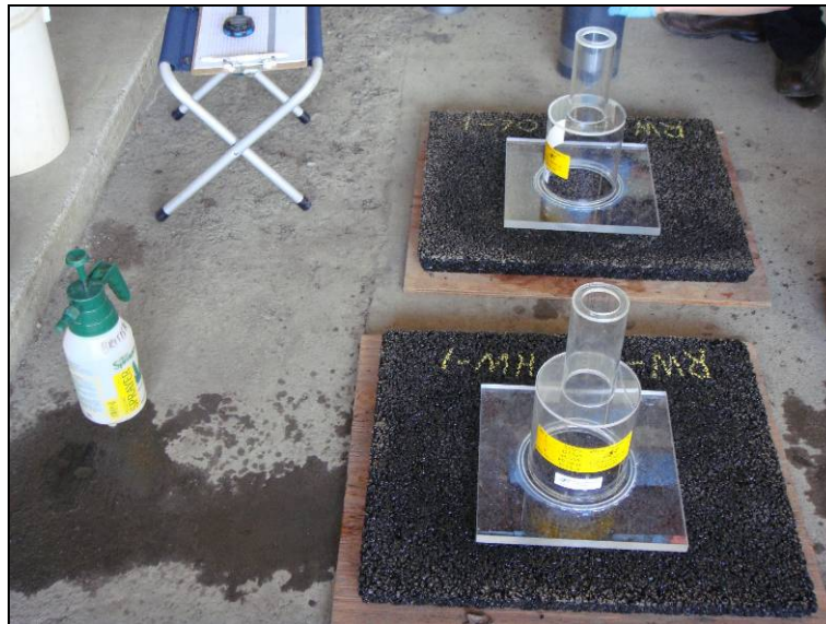
Figure 7.1: Permeability testing on compacted slabs.
