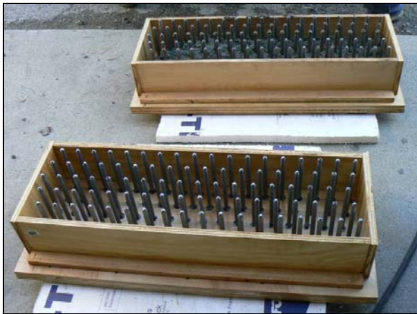
Figure 6.7: Precast beam specimen molds.
