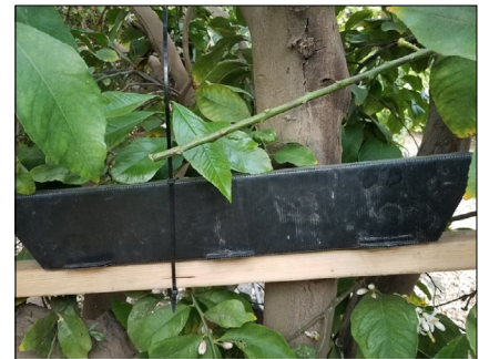
Plate I. Tracking tunnel attached to a 3-foot section of a 2-inch-by-4-inch wooden board. Tracking tunnels are used to monitor roof rat presence. Source: Roger Baldwin, UC Davis.
