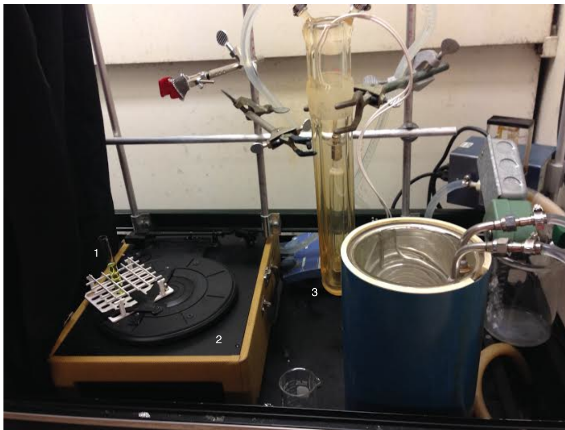
Figure 3.17. Photochemical experimental setup for irradiation of NMR reactions (1: borosilicate test tube with 2 mM aq. K_2CrO_4 , 1% w/v K_2CO_3 optical solution; 2: turntable; 3: 450 W Hanovia Hg vapor lamp).
