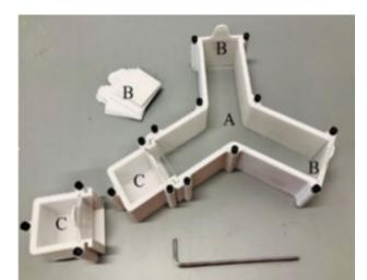
Note. A is the 3D-printed maze, B are the removable color panels, and C is the bee containment box.
