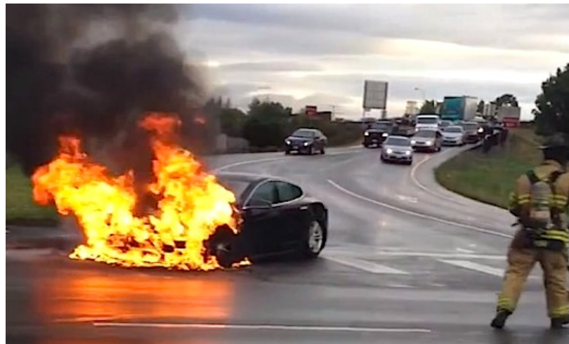
Figure 1.2: Tesla Model S battery fire in Washington State in 2013 [4].
