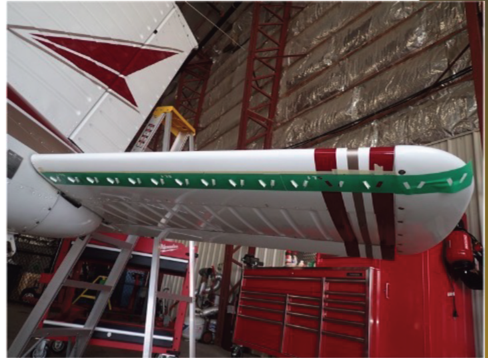
Piper PA-28-180 Test Aircraft (N4859L) VG Installation on Horizontal Stabilator
