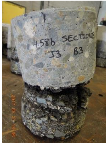
b) Asphalt crushing / debonding at corners
