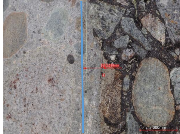
b) Type II/V cement on top of milled HMA, depth of penetration of 2.29 mm (0.09 in.).
