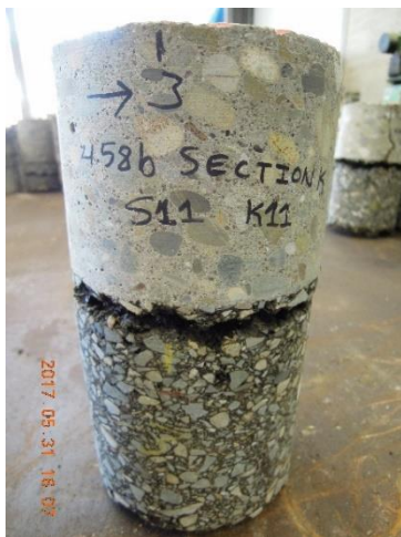
d) Band delamination around 3.6 x 3.6 m (12 x 12 ft) slab perimeter
