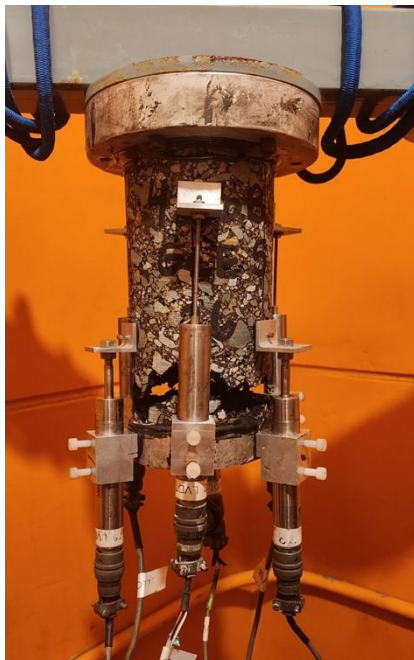
a) Hanging test setup
