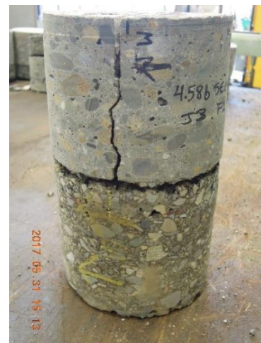
c) Asphalt cracking below the transverse joint
