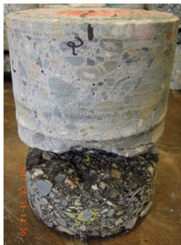
b) Asphalt crushing / debonding at corners
