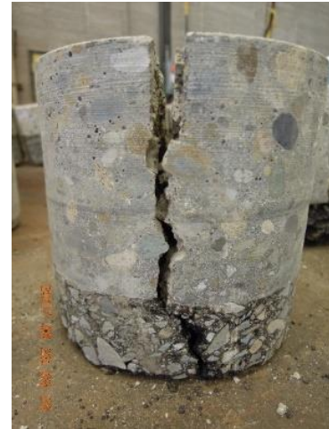
c) Asphalt cracking below the transverse joint
