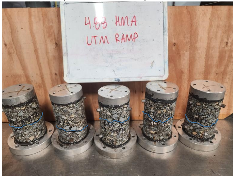
b) HMA tensile ramp failures
