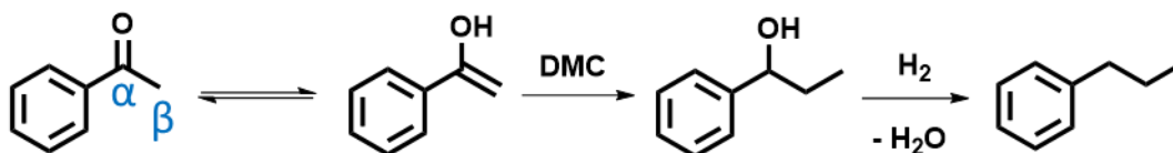
Scheme 2.4. Plausible mechanism for the β-carbon methylation of 1-phenylethanol to form propylbenzene. Acetophenone tautomerizes to the enol 1-phenylethen-1-ol. DMC = dimethyl carbonate.
