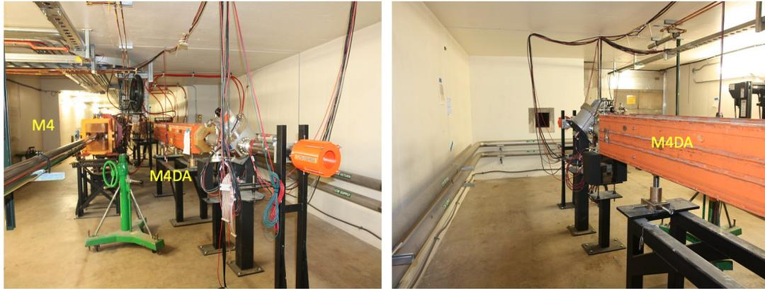
Figure 9.13: Location of the M4 diagnostic absorber (M4DA) relative to the M4 line, which contains the extinction components including the AC Dipole [13].
