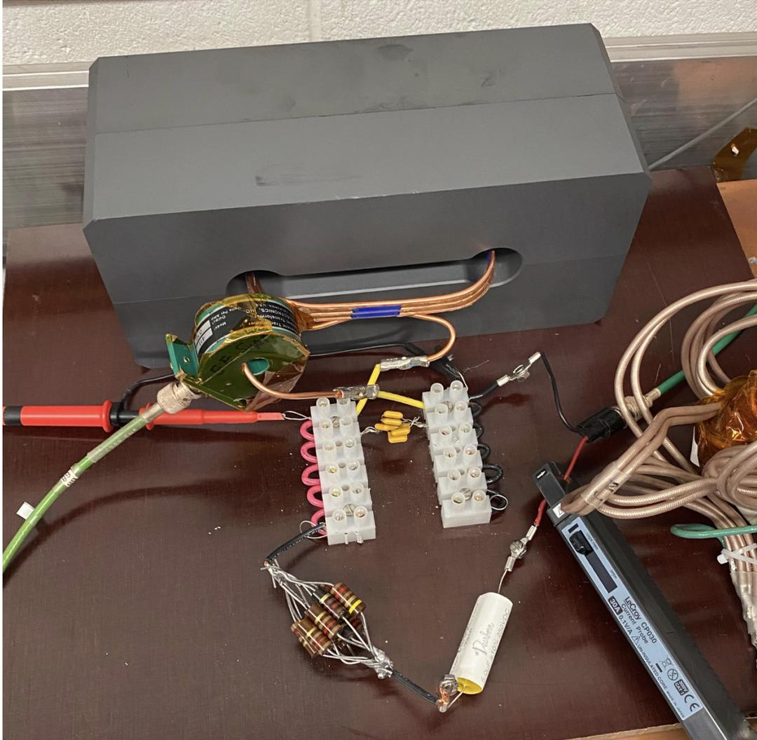
Figure 8.2: Overview of “dipole mode” circuit setup for ferrite characterization. A voltage, and two current probes in conjunction with an oscilloscope are used to measure the voltage across the capacitor bank, the current through the copper coil and the current into the circuit respectively.
