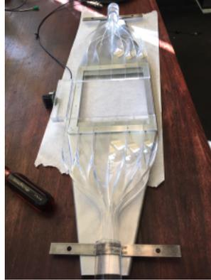
Figure 9.4: Picture of the T0 detector [21].
