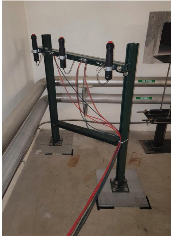
Figure 9.14: The Upstream Extinction Monitor (UEM) prototype arm with mounted PMTs attached to quartz crystals [13].
