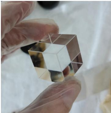
(a) Square quartz crystal that will be used to detect charged particles for a beam profile measurement [13].
