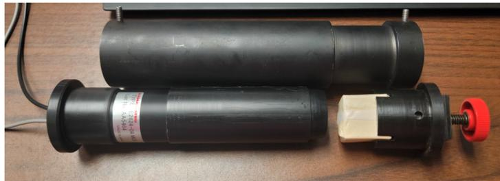
(b) PMT setup with metallic housing and quartz crystal mounted to an endcap. The item in the top of the picture is the metallic housing that will surround the PMT and the PMT with endcap is the bottom left item. The object on the bottom right is the had wrapped Tyvek crystal holder attached to an endcap [13].
