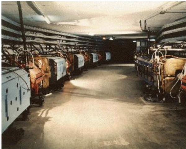
Figure 5.5: Picture of the Debuncher (outer ring) and the Accumulator (inner ring) [12].
