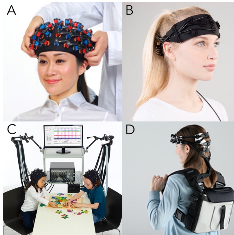
Figure 2 – Examples of fNIRS head layouts and machines from various production companies. A) High density, full brain coverage with the ETG-4000 unit from Hitachi ( hitachimed.com ). B) A lightweight, prefrontal-specific layout with the OctaMon unit from Artinis ( artinis.com ). C) A hyperscanning study imaging multiple concurrent participants with the NIRScout unit from NIRx ( nirx.net ). D) Backpack design of the mobile LIGHTNIRS unit from Shimadzu ( shimadzu.com ).
