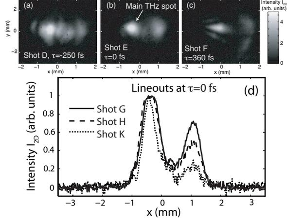
FIG. 3: Three characteristic single-shot 2D THz images  $I_{2D}(x, y, \tau)$ , taken at different values for the delay between the THz and laser pulse: (a)  $\tau = -250$  fs, (b)  $\tau = 0$  fs, and (c)  $\tau = 350$  fs. At a fixed delay  $\tau = 0$  fs, lineouts at  $y = 0$  of three consecutive shots are displayed in (d).
