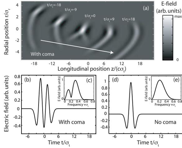
FIG. 4: (a) Evolution the simulated field profile  $E(r, z)$  at various time steps. The  $90^\circ$ -off-axis parabola was rotated by  $0.4$  rad (coma). With coma present, the temporal field profile  $E(t)$  at a fixed location  $r/\sigma_r = -1$  and  $z = 0$  is shown in (b), with the Fourier transformation  $|E(\nu)|$  in (c). For comparison, without coma present, the field profiles  $E(t)$  and  $|E(\nu)|$  at the center of the focal spot are shown in (d) and (e), respectively.
