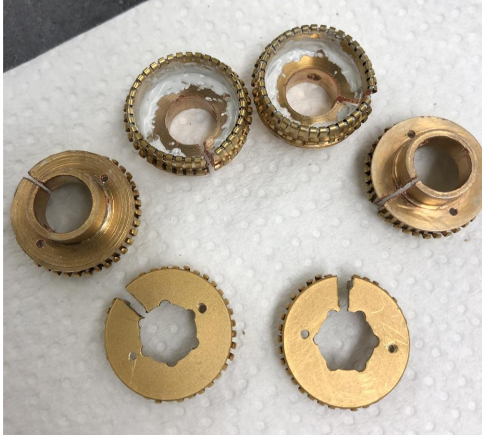
Fig. 3.2: Home-made contact baffles that are crucial to reduce the heat load into PPMS sample chamber. They work as both contact baffles between the probe and the PPMS sample chamber, and radiation shields to reduce thermal radiation from the top.
