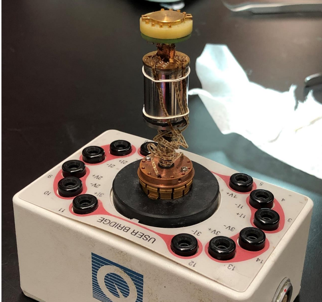
Fig. 4.3: Picture of the ADR unit sitting on a PPMS user bridge, the paramagnetic salt is in the stainless-steel container, container is connected to the bottom puck through the carbon fiber rod.
