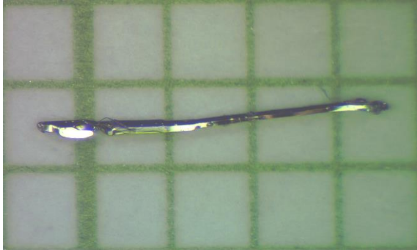
Fig. 3.6: A \text{NiBi}_3 crystal used in this study, it is needle shaped with shiny but curvy surfaces.
