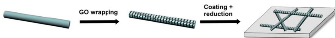
Figure 1. Schematic illustration of the graphene oxide wrapping, film deposition, and reduction process to fabricate the transparent nanowire conducting films.
