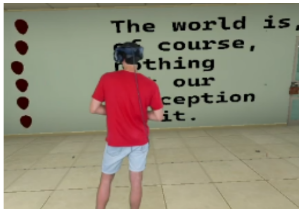
(b) Environment designed to reveal headset refresh rate via perceived motion differences.
