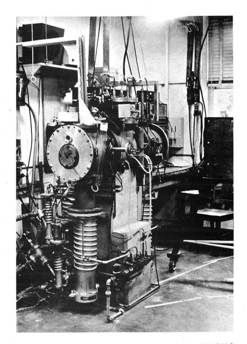
Fig. 11. The atomic beam apparatus as seen from the oven end.
