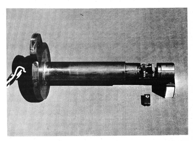
Fig. 6. The resistance heated oven loader assembly.
