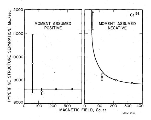
Fig. 32.  $\triangle v$  sign curves for  $Cs^{132}$ .
