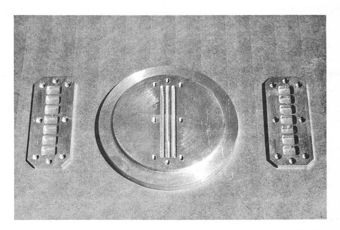
Fig. 21. The powder cyclotron target.
