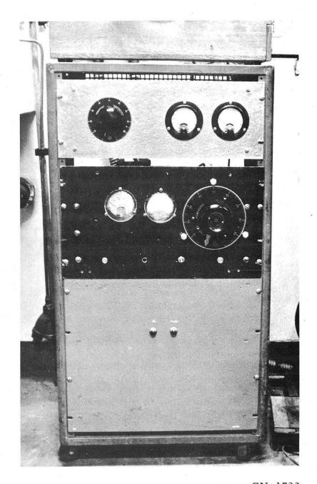
Fig. 10. The 1000 v, 500 ma electron bombardment power supply.
