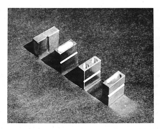
Fig. 24. The sulfur coated buttons used to collect radioactive cesium atoms.
