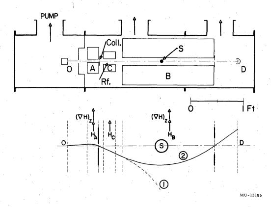
Fig. 5. Schematic arrangement and trajectory in an atomic beam, flop-in apparatus.
