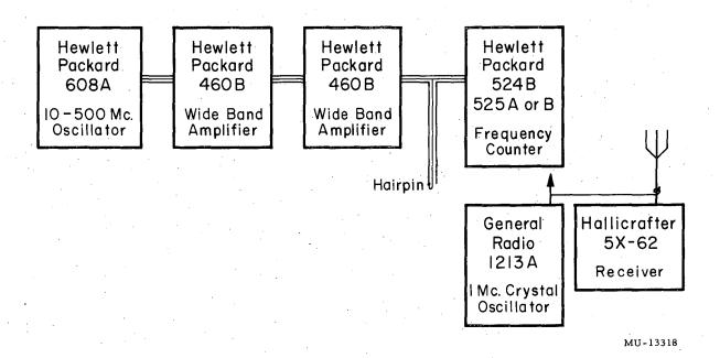
Fig. 16. Radiofrequency equipment (10 to 200 megacycles per second)
