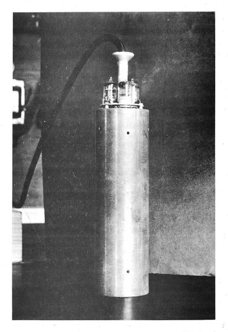
Fig. 18. An assembled X-ray scintillation counter.
