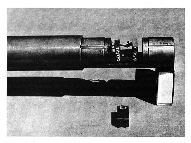
Fig. 7. The resistance heated dry dock assembly.
