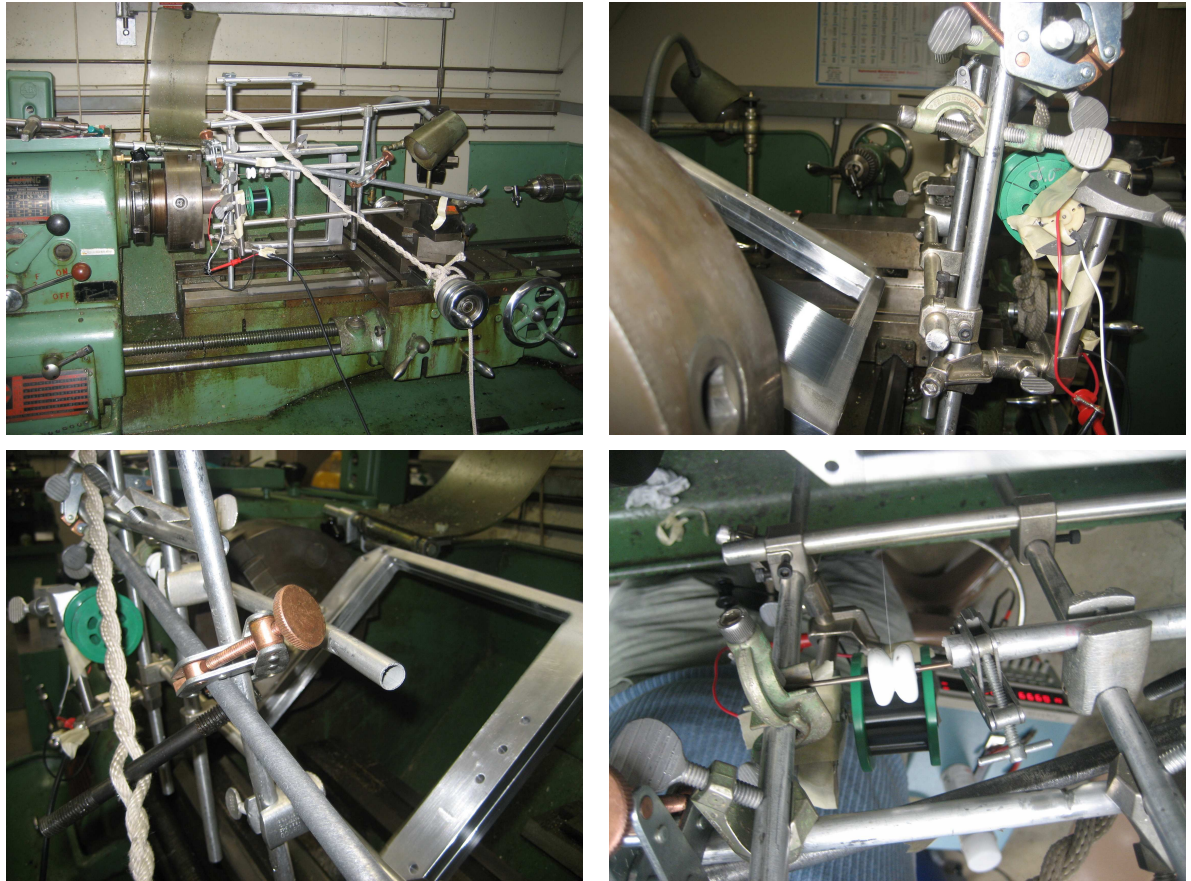
Figure 3.2: Pictures showing the setup to wind the wire grids for the UCSD FTS. The empty grid frames are mounted into the lathe using an adapter, and as the lathe turns, the cross guide moves the grids longitudinally at the desired rate for a given wire spacing. The spool feed is a home-made ceramic piece designed to smoothly guide the wire from the manufacturer's spool on to the wire grid. The spool is reverse biased with a DC motor to provide the correct level of tension.
