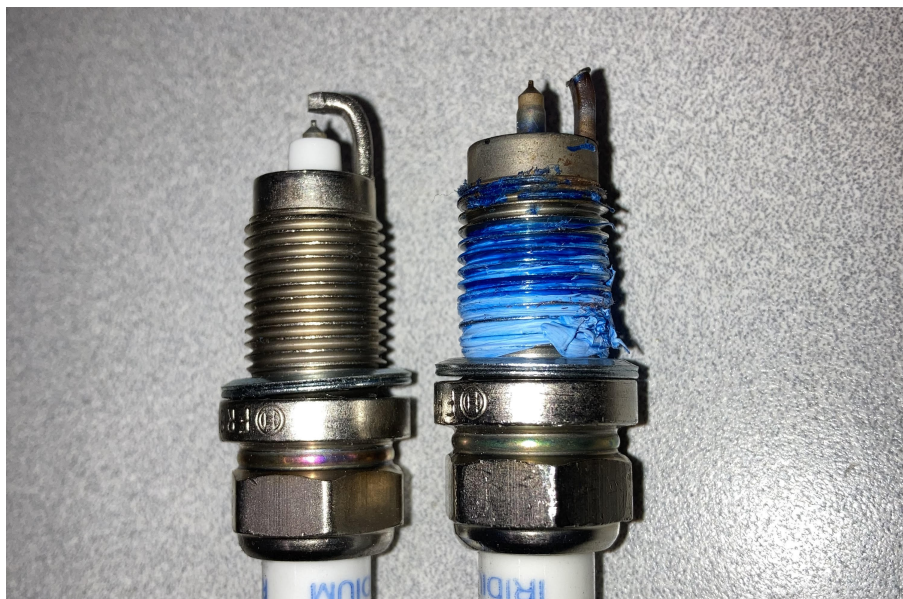
Figure 6.7. New (left) vs Used (right) Spark Plug
