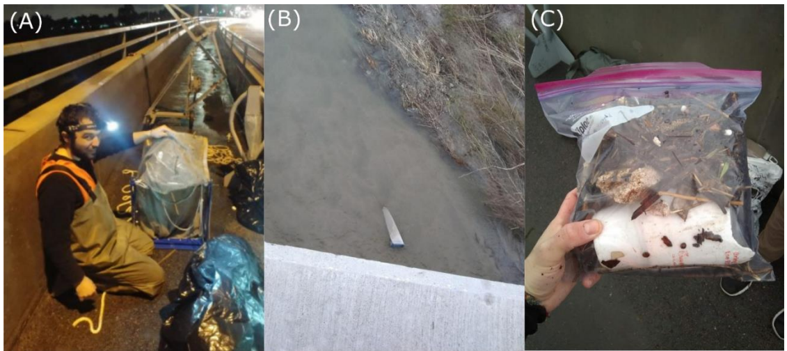
Figure 4-2: A) Sample collection apparatus and B) deployment from a bridge. The net has a 400 mm square aperture and a 5 mm mesh. C) An example of a sample that will be sorted for plastic visually.
