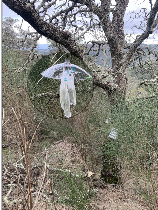
Figure 2. Transplantation Method. A photo of the method used for the transplantation experiment. Each site had a shield with 4 bags of lichens hanging from it.
