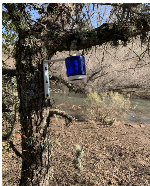
Figure 4. MerPas Methods. A photo showing the setup of the air collectors. Near each shield, 2 collectors were installed approximately 1.5 m from the ground.
