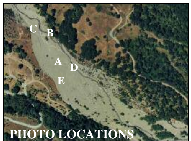
Figure 10: Remnants of Channel Reconstruction Project. A) Abandoned channel B) Suspected remnants of rock and log revetment; C) Suspected remnants of vortex rock weir; D) Active channel looking downstream; E) Vertically placed logs in floodplain that are remnants of debris flow regulation structures.
