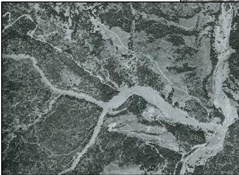
Figure 2: Changes in Cuneo Creek Channel Configuration (1942-1965). Upper photograph is from 1941 prior to extensive logging. Middle photograph is from 1964, after extensive logging and channel aggradation due to 1955 flood. Lower photograph is from 1965 after further logging and shows extreme channel aggradation due to 1964 flood.
